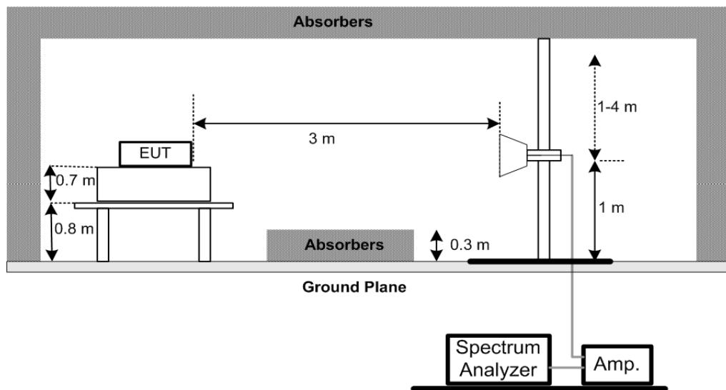
(C) For radiated emissions below 30MHz
