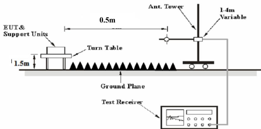
The radiated emission tests were performed in the 3 meters Chamber A, using the setup accordance with the ANSI C63.10-2013. The specification used was the FCC 15.209, 15.205 and FCC 15.249 limits.
