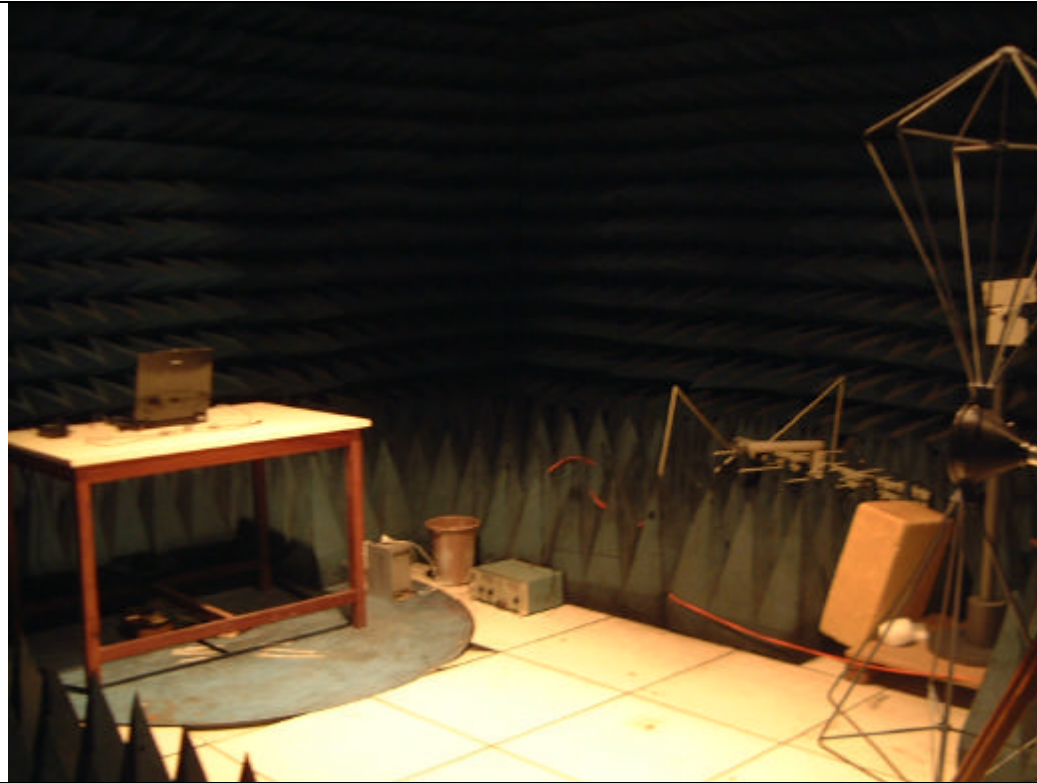
Radiated Emission test setup 30MHz - 230MHz
