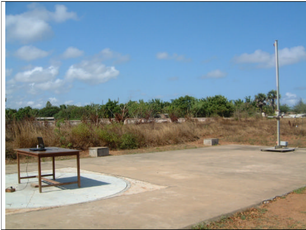
Radiated emission test setup Horizontal polarization.
