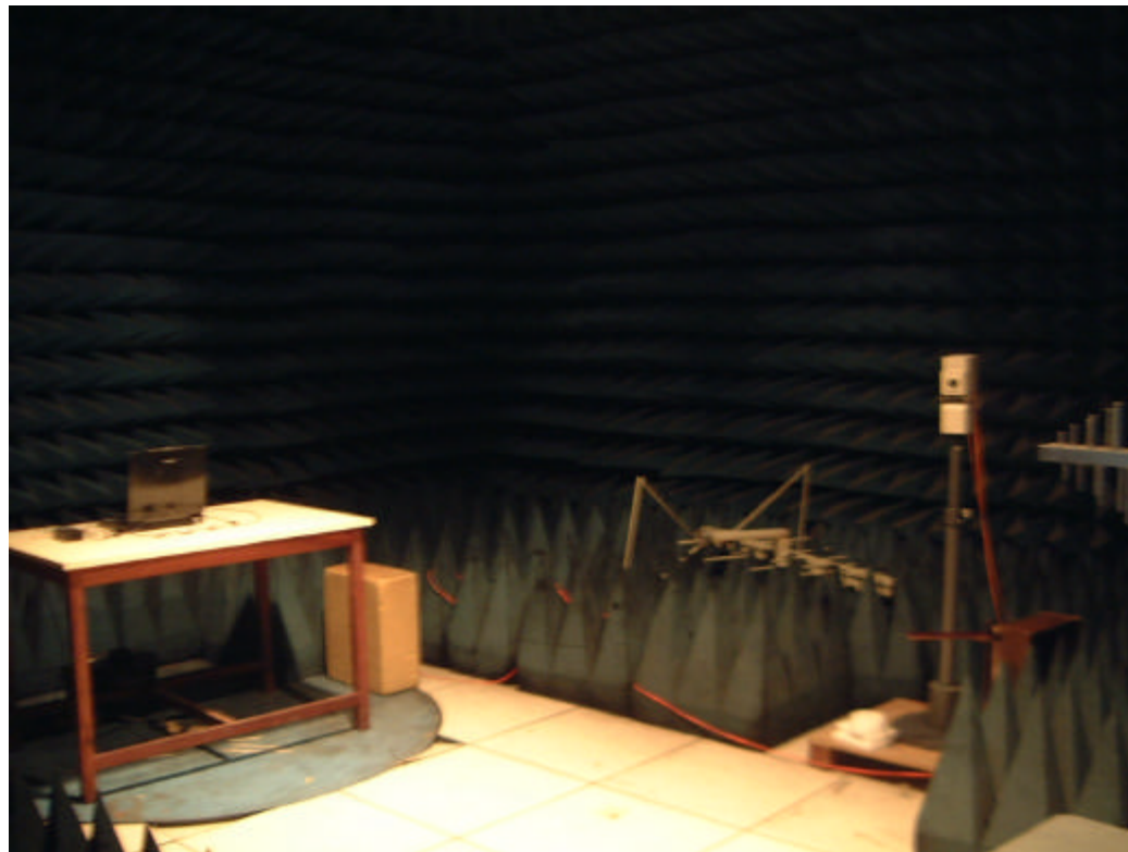
Radiated emission test setup 230MHz -1GHz)
