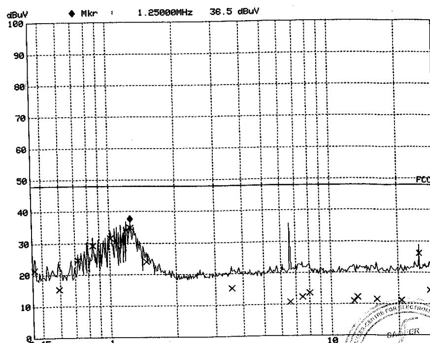
Conducted Emission QP Band Width: 9KHz: Plot 1A
