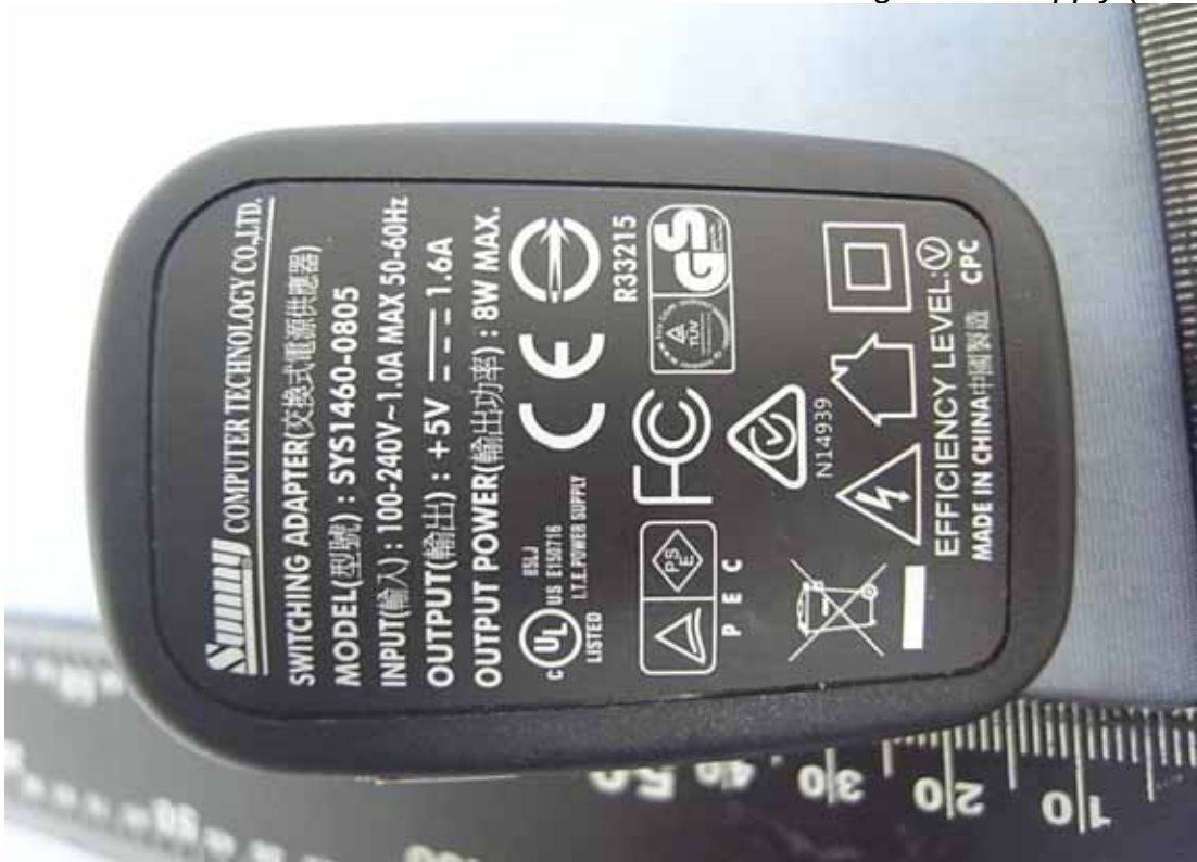
Figure 7 Switching Power Supply (Label View)
