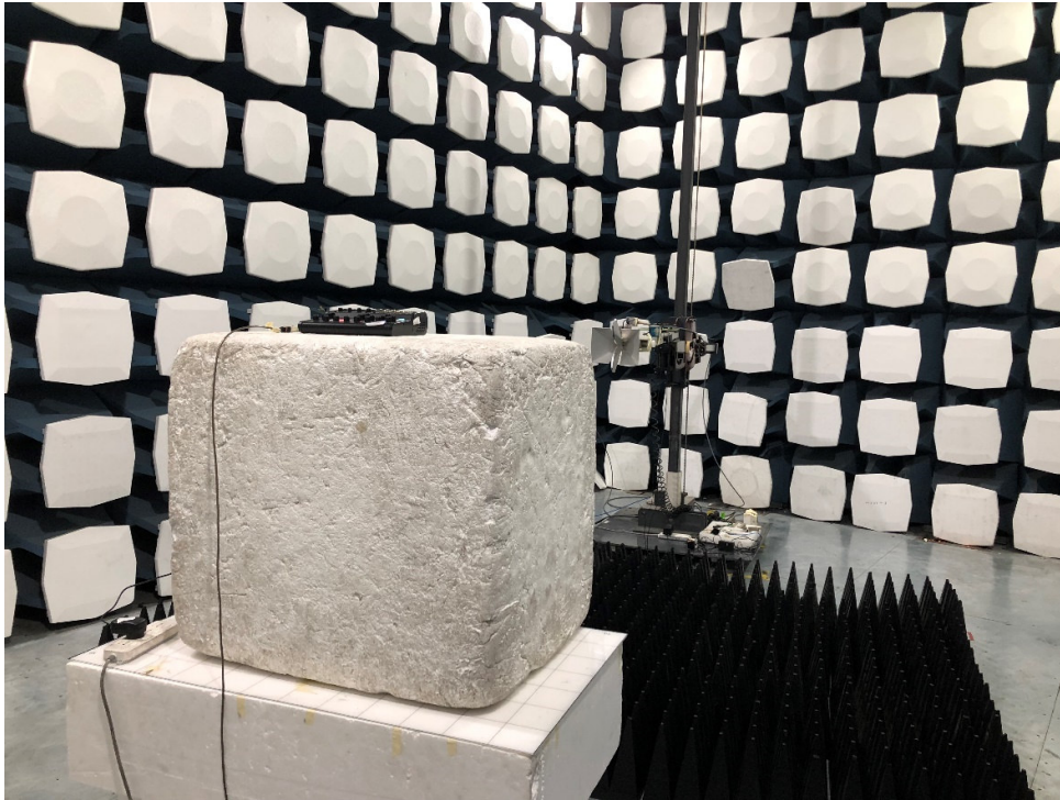
Picture 1 Radiated Emission Test Setup
