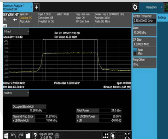
Band41-20MHz-QPSK-41490-100RB#0
