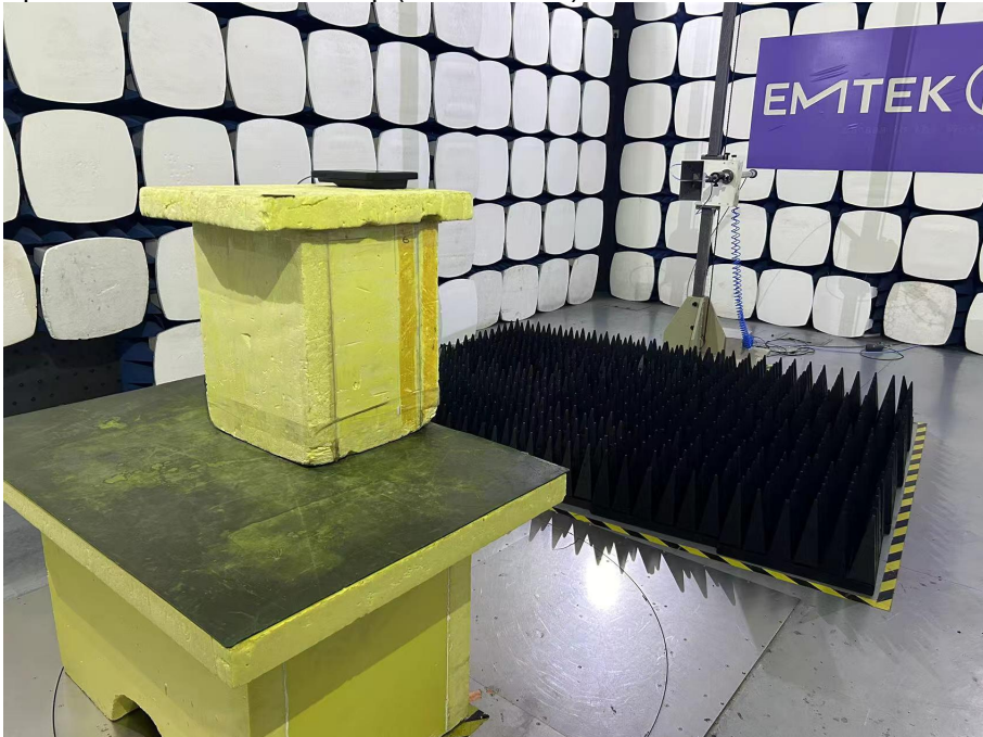
Spurious Emission Test Setup (Above 1GHz)
