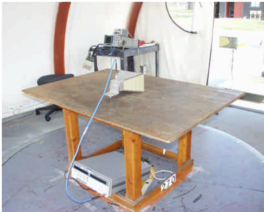
1 – 18 GHz Substitution Method Setup
