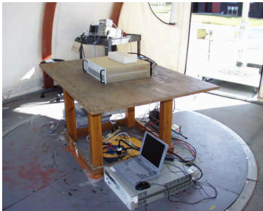
1 – 18 GHz Radiated Emission Setup
