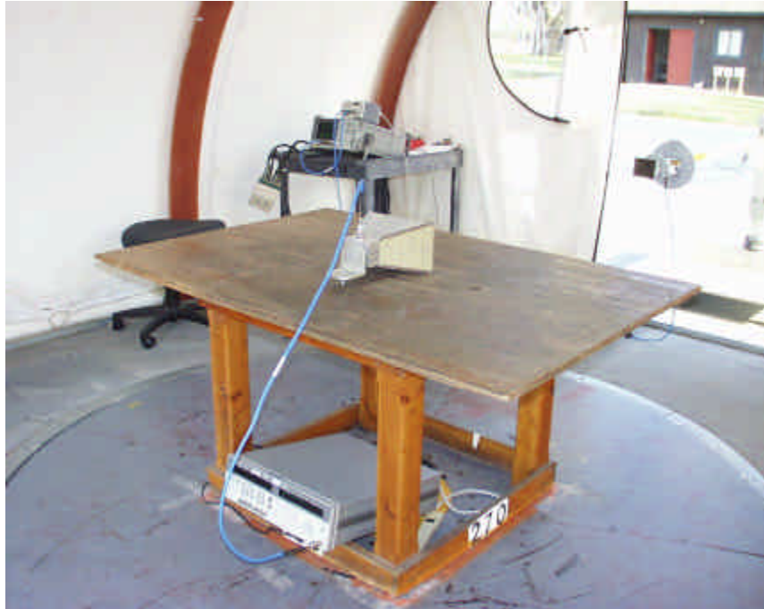
18 – 20 GHz Substitution Method Setup
