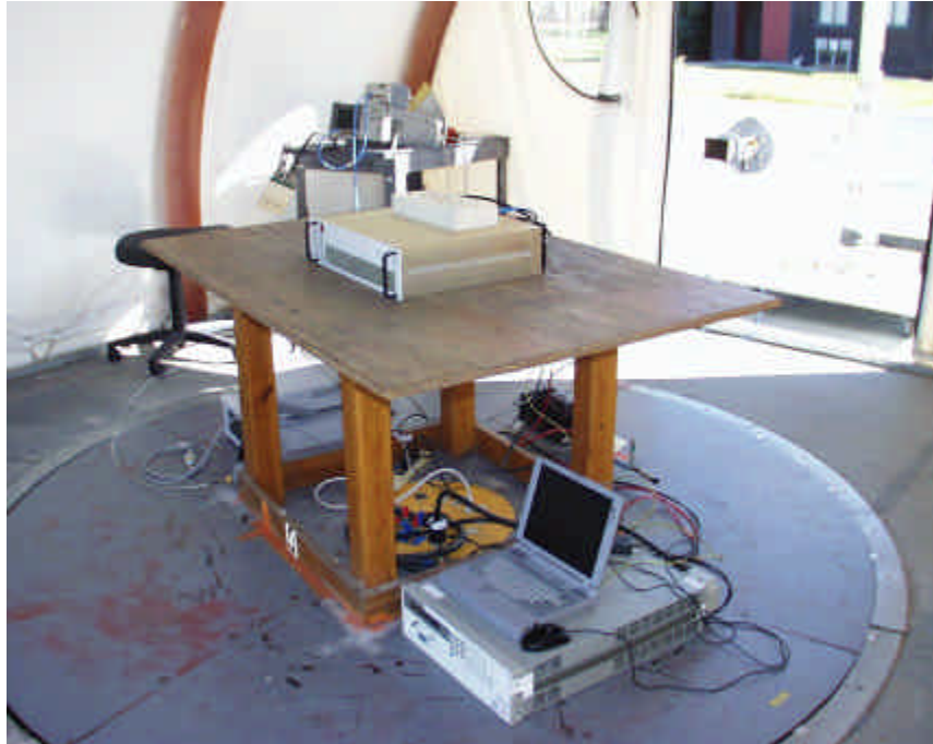
18 – 20 GHz Radiated Emission Setup
