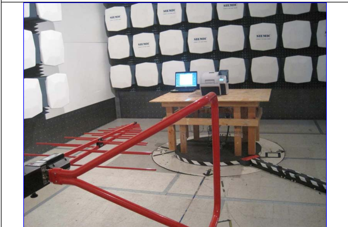
Radiated Emission Test Setup (30M-1GHz) - Front View
