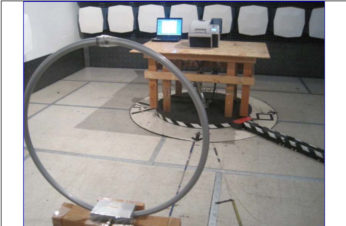
Radiated Emission Test Setup (below 30MHz) - Front View
