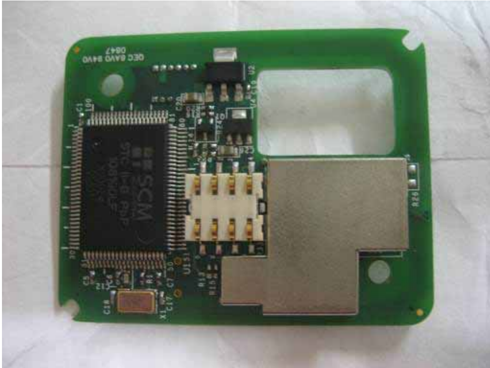
Contactless RFID Board with shielding –Bottom View
