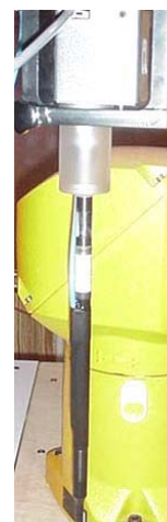
ET3DV6 E-Field Probe
