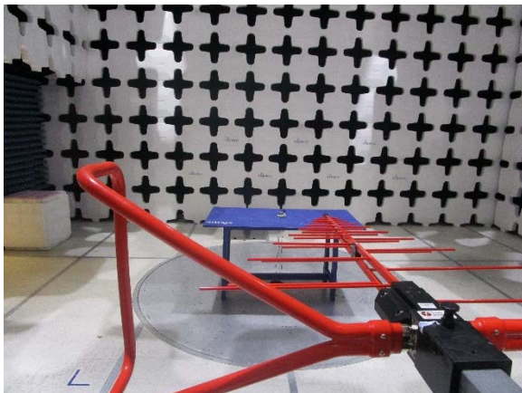
Radiated Emission Test setup (<1GHz) – Front View
