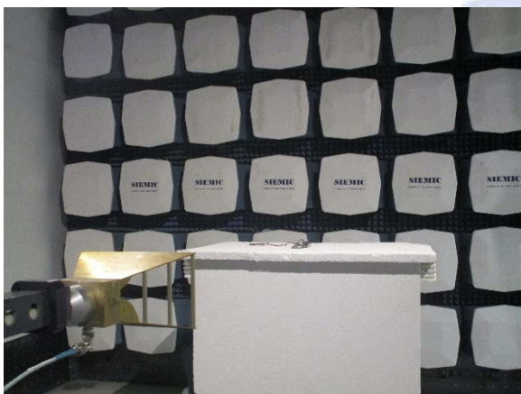
Radiated Emission Test setup (>1GHz) – Front View
