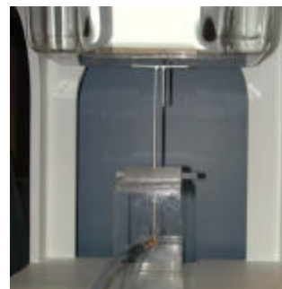
Figure A.1 Dipole Validation Test Setup
