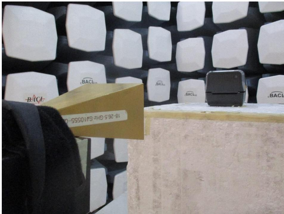
**1.6 18 – 26.5 GHz at 1 Meter Rear View**
