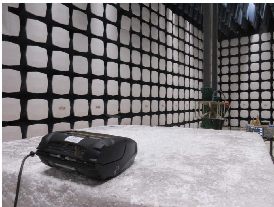
**1.7 18-26.5 GHz at 1 meter- Front View**
