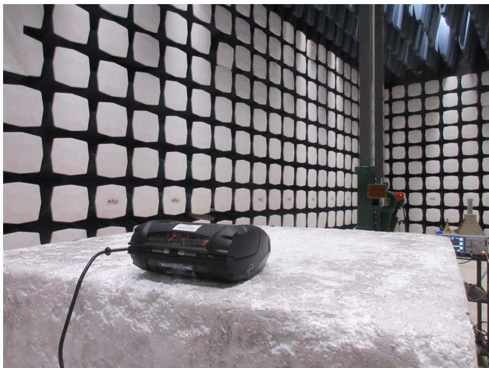
**1.9 26.5-40 GHz at 1 meter- Front View**
