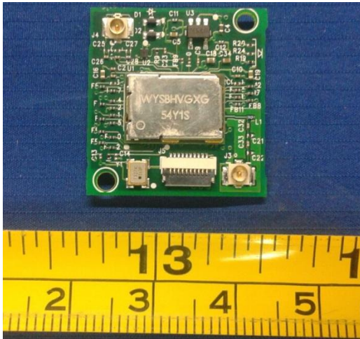
EUT Radio with Shielding Top View
