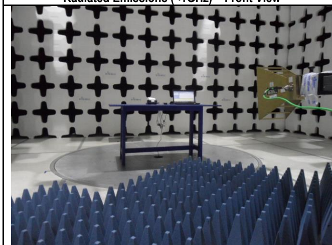
Radiated Emission Test Setup (>1GHz) - Front
