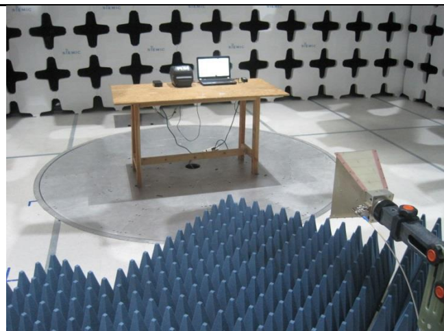
Test setup at 3 meter distance (>1GHz) - Front
