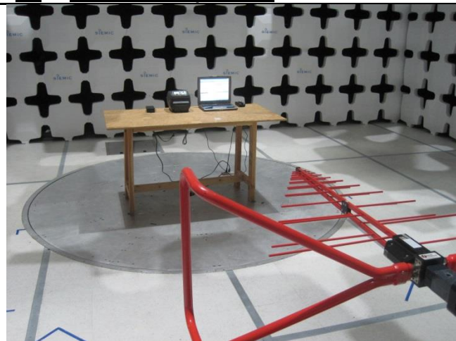
Test setup at 3 meter distance (<1GHz) - Front
