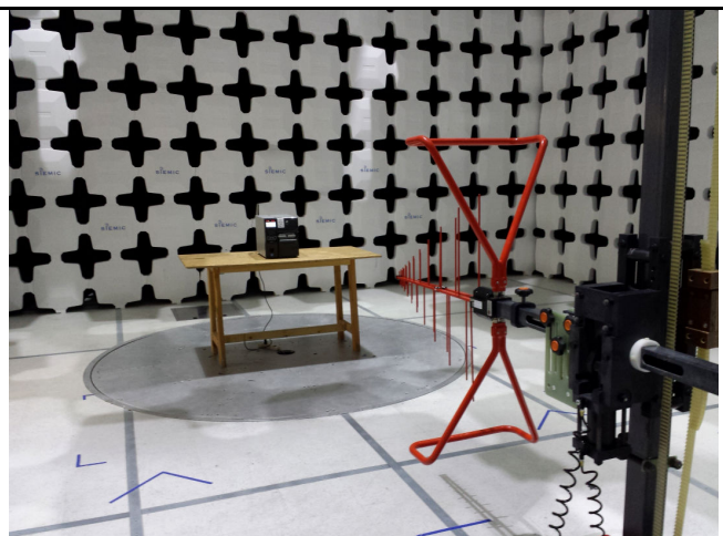
Radiated Emission below 1GHz – ZT410 (Rear)
