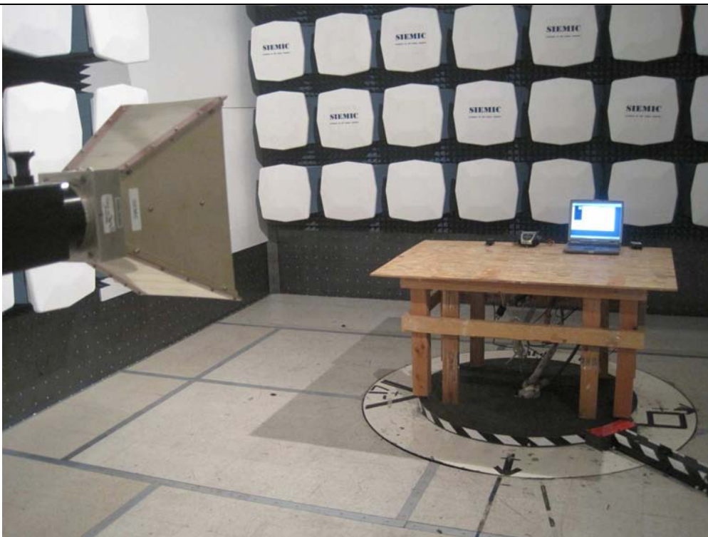
Radiated Emission Test Setup (Above 1GHz) - Front View
