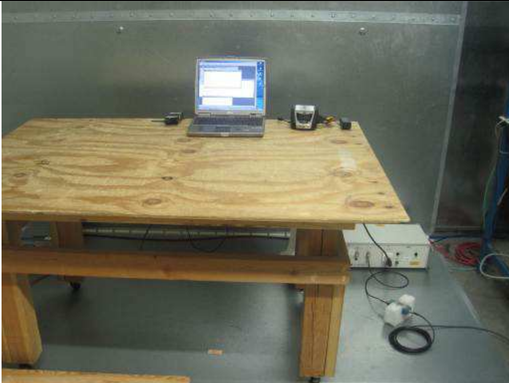
Conducted Emission Test Setup – Front View
