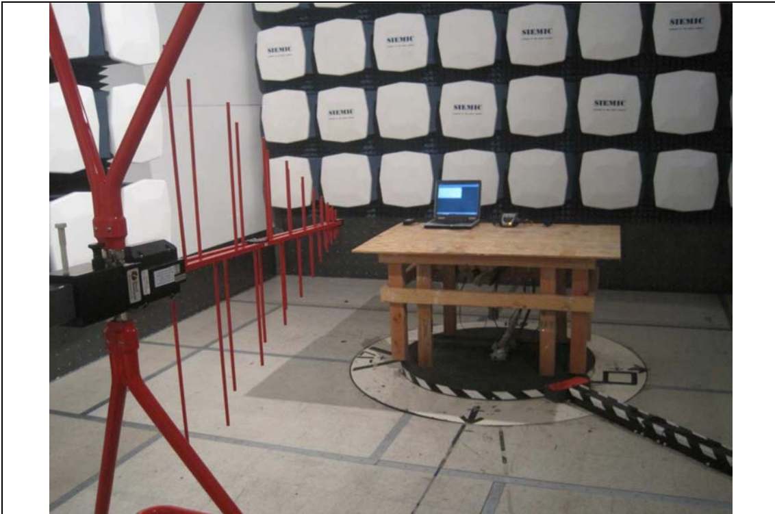
Radiated Emission Test (30MHz – 1GHz) - Front View
