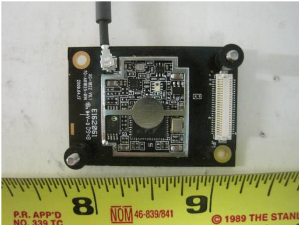
Radio Board shielding off View
