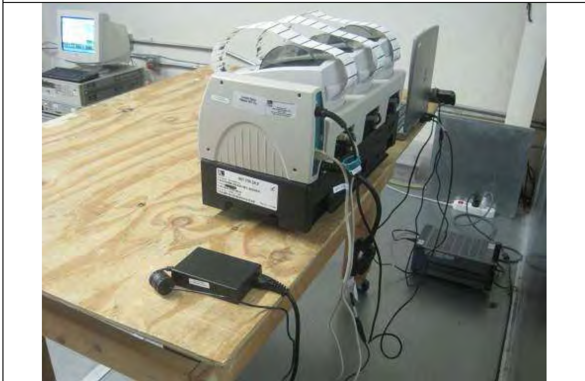
Conducted Emission Test Setup – Rear View
