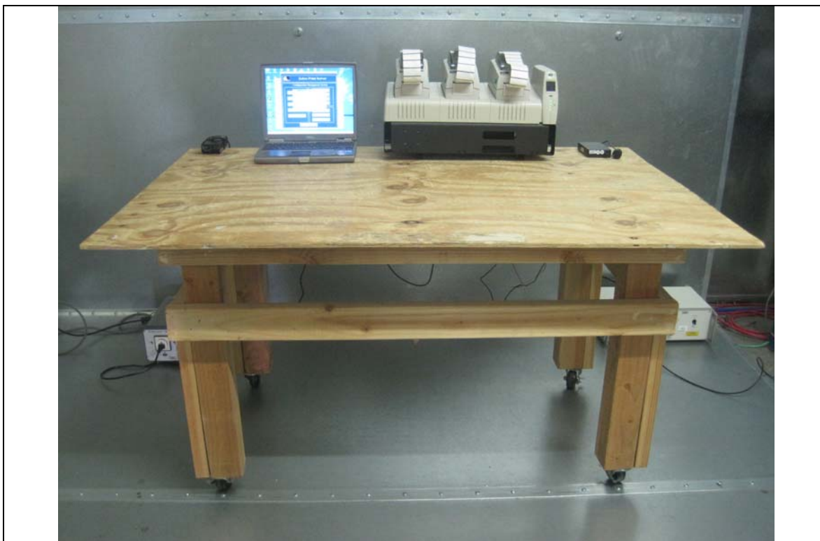
Conducted Emission Test Setup – Front View
