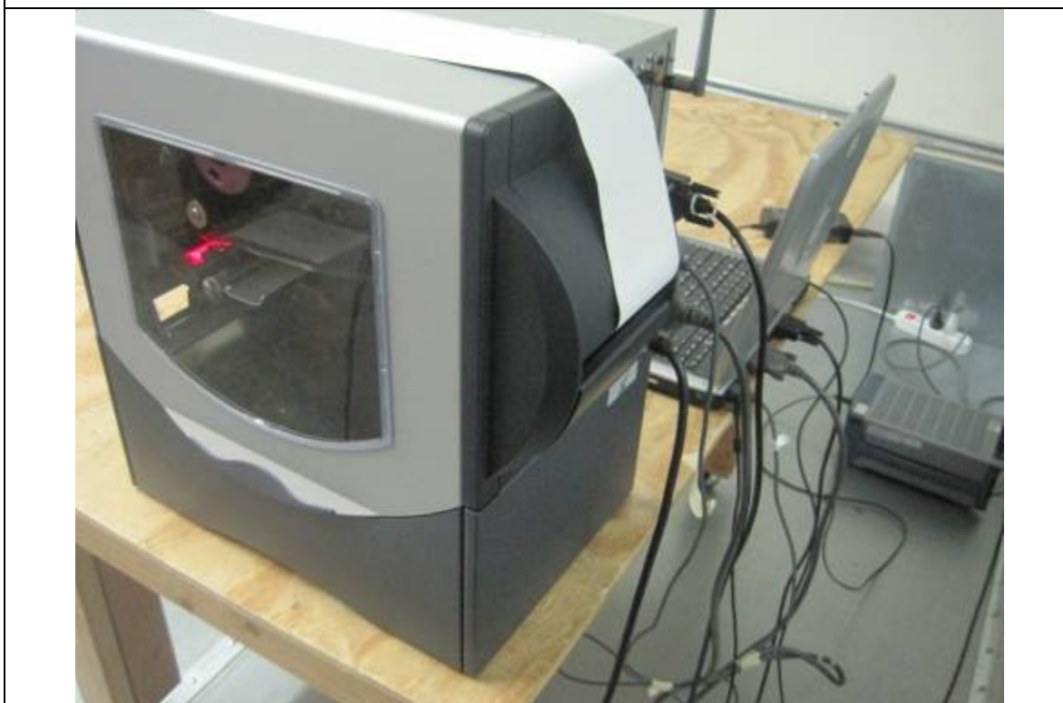
Conducted Emission Test Setup – Rear View
