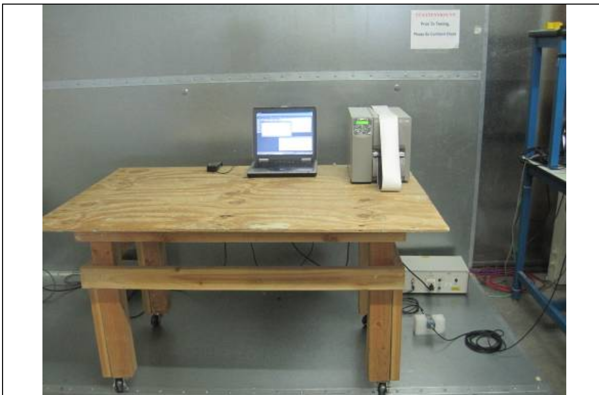
Conducted Emission Test Setup – Front View
