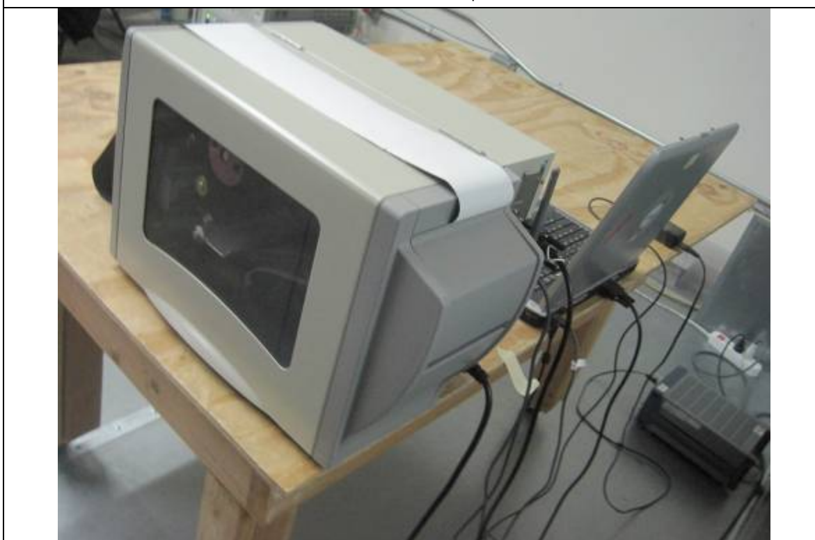
Conducted Emission Test Setup – Rear View
