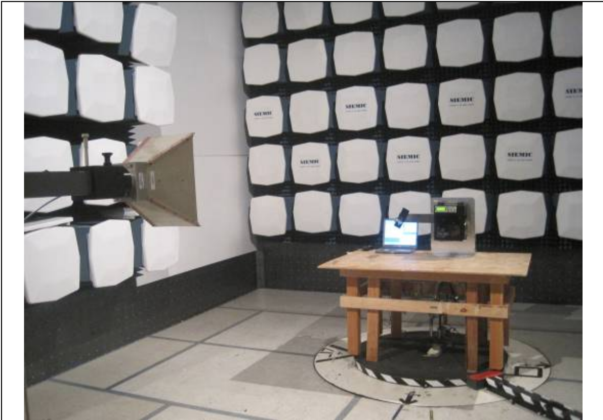
Radiated Emission Test Setup (below 1GHz) - Front View
