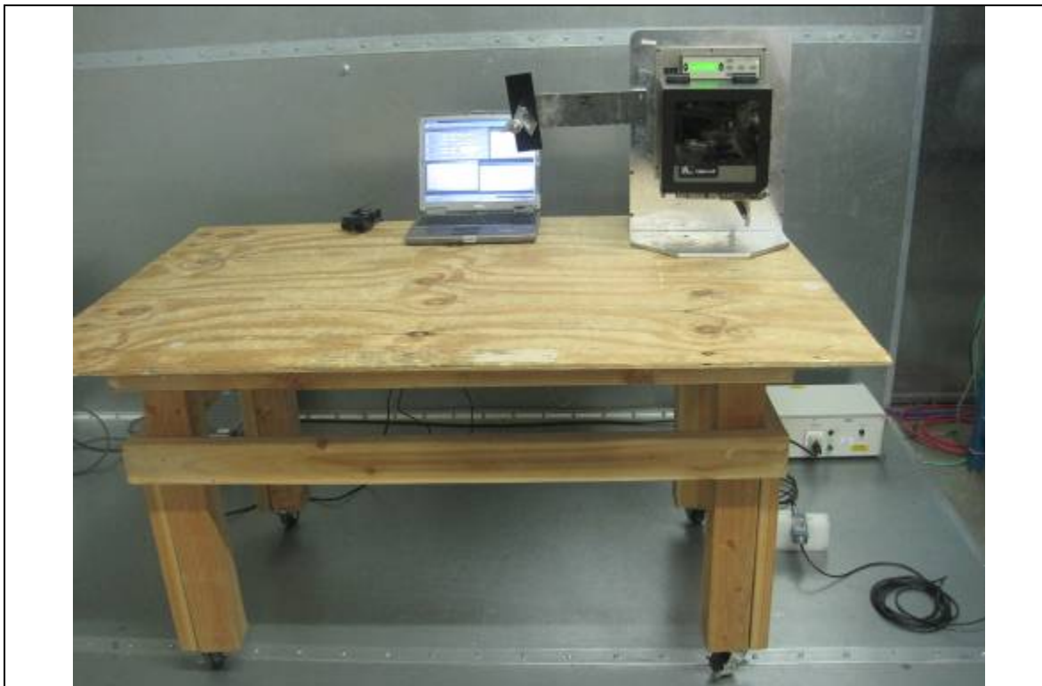
Conducted Emission Test Setup – Front View
