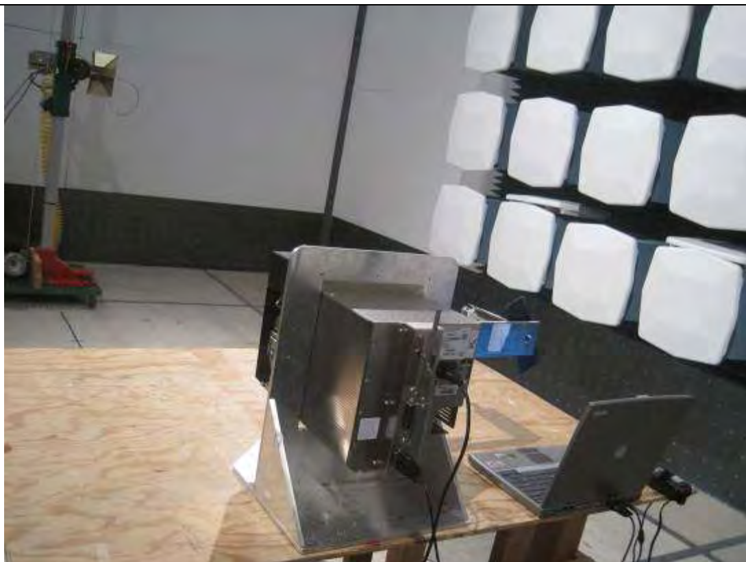
Radiated Emission Test Setup (above 1GHz) – Rear View
