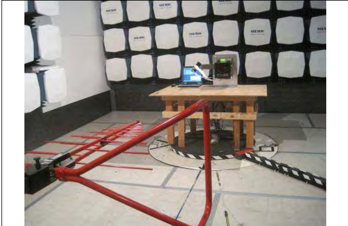
Radiated Emission Test Setup (below 1GHz) - Front View
