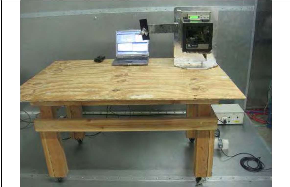
Conducted Emission Test Setup – Front View
