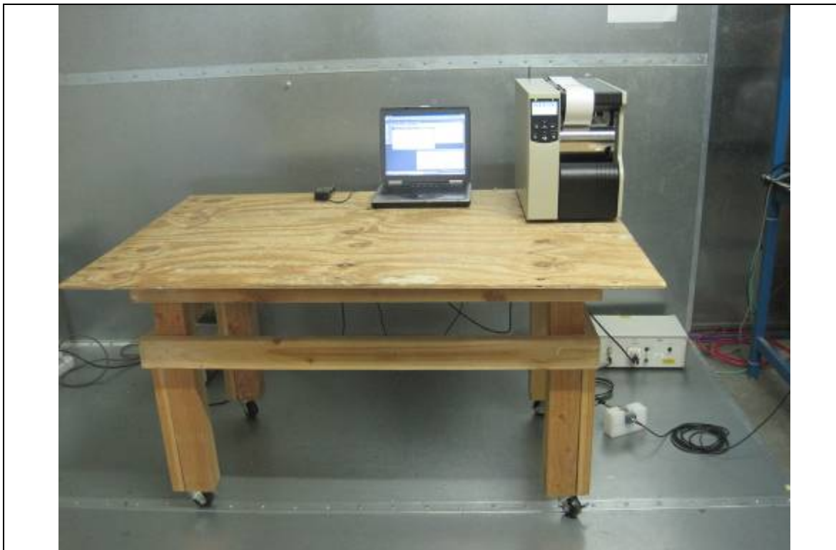
Conducted Emission Test Setup – Front View
