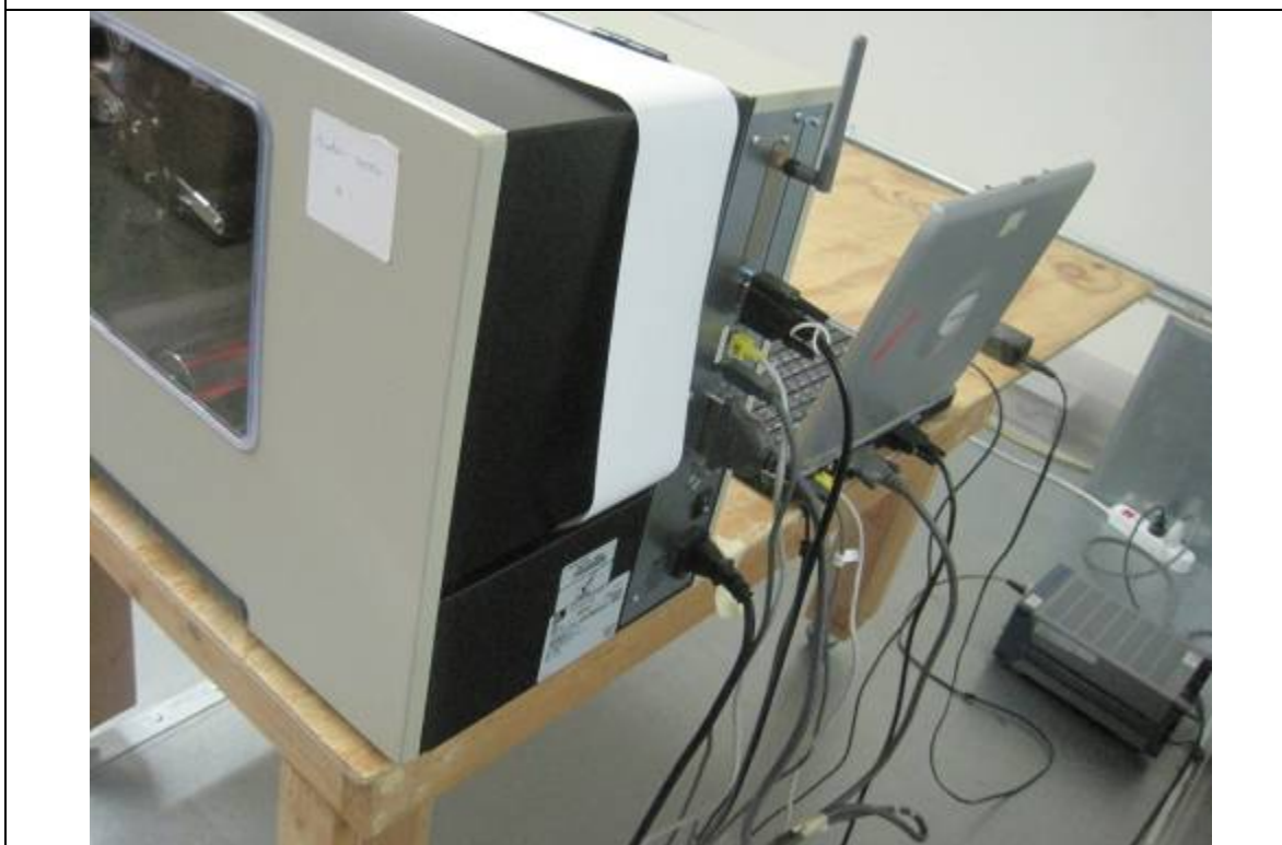
Conducted Emission Test Setup – Rear View
