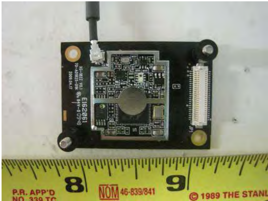
Radio Board shielding off View
