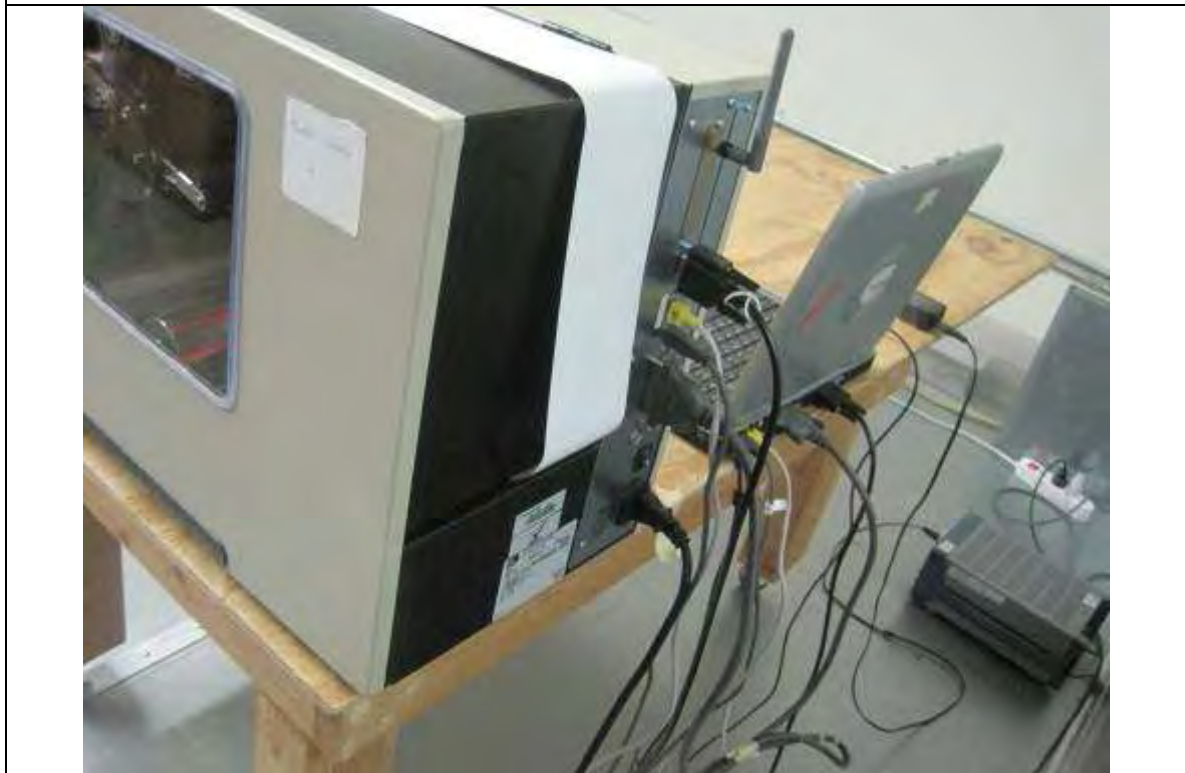
Conducted Emission Test Setup – Rear View
