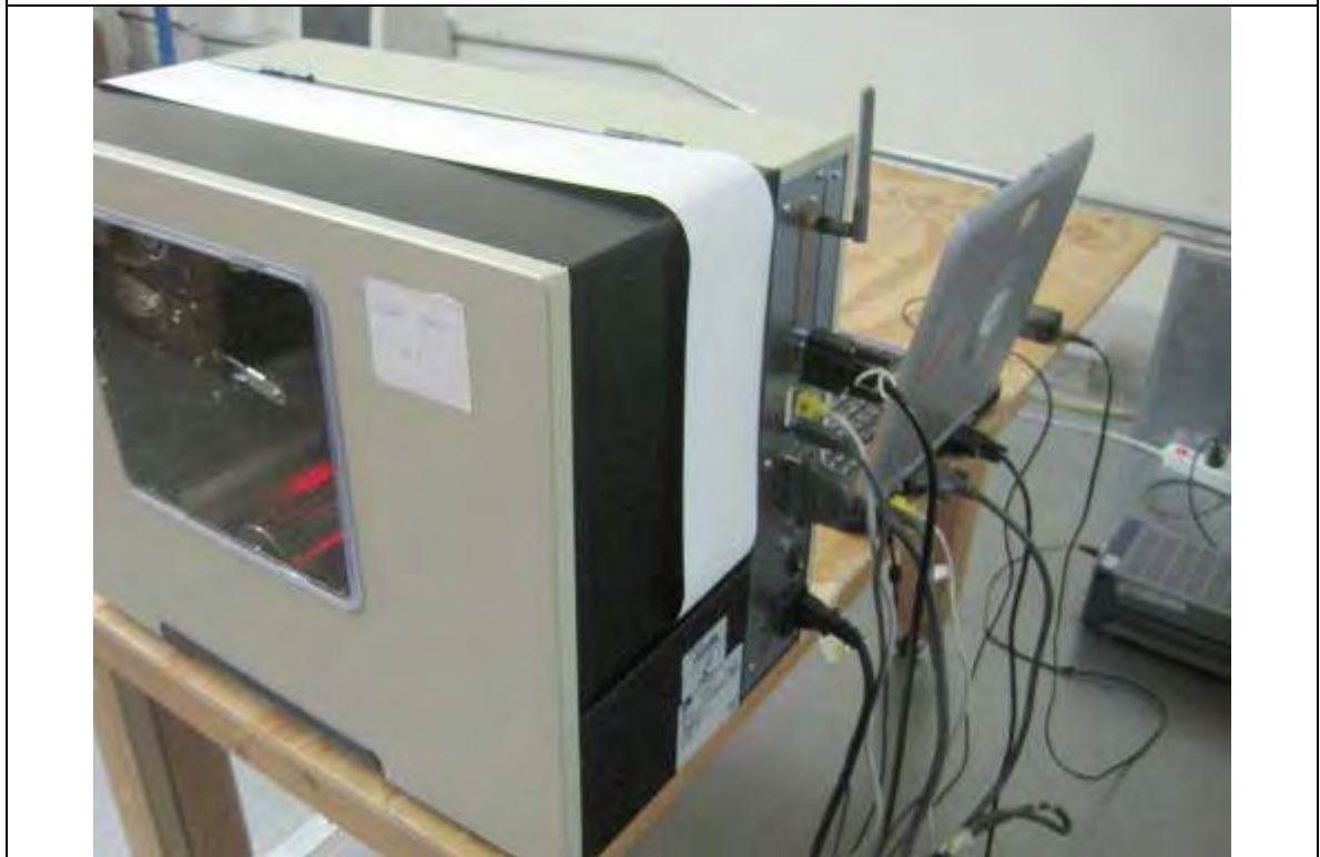
Conducted Emission Test Setup – Rear View
