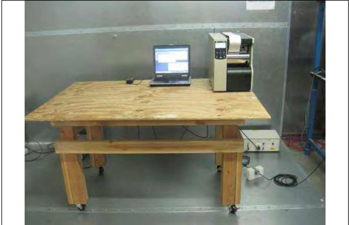
Conducted Emission Test Setup – Front View
