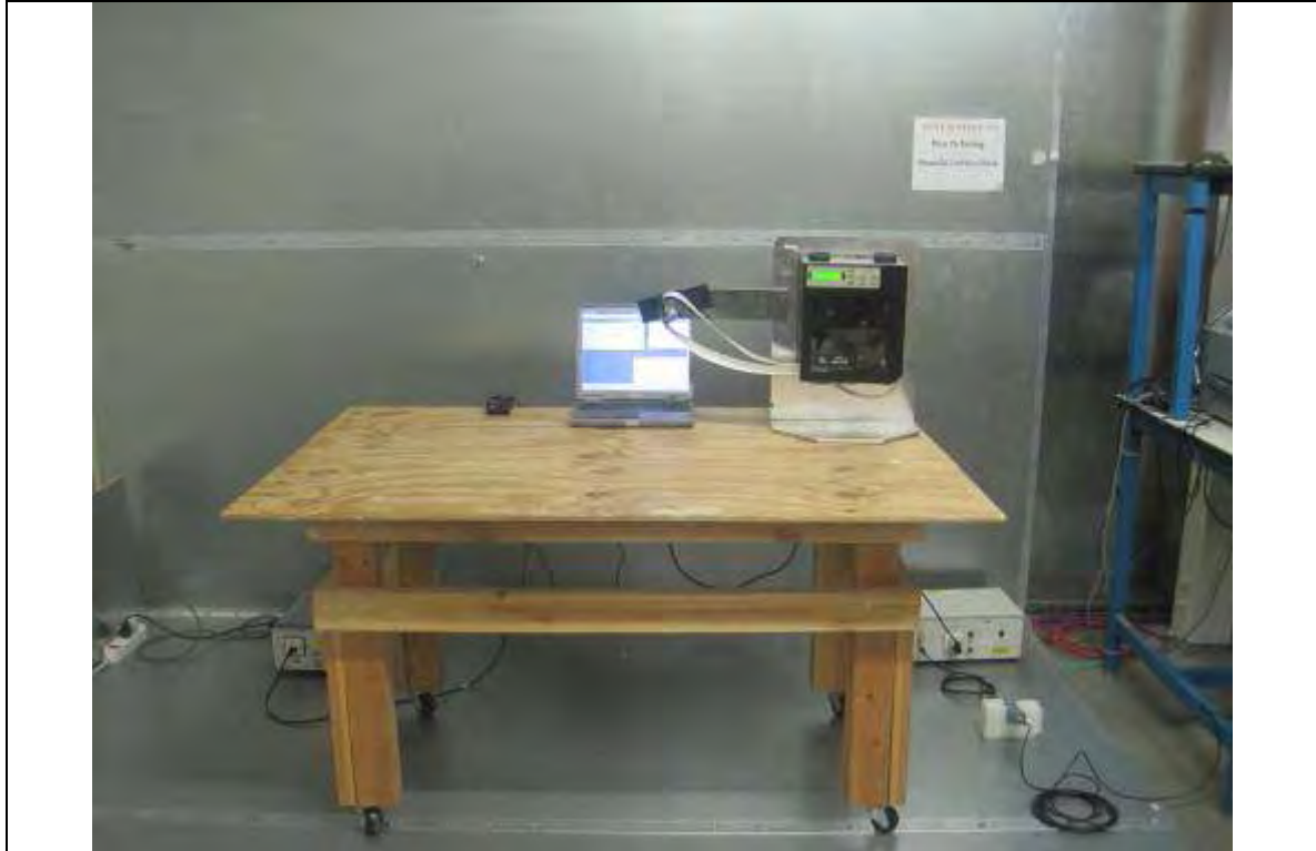
Conducted Emission Test Setup – Front View
