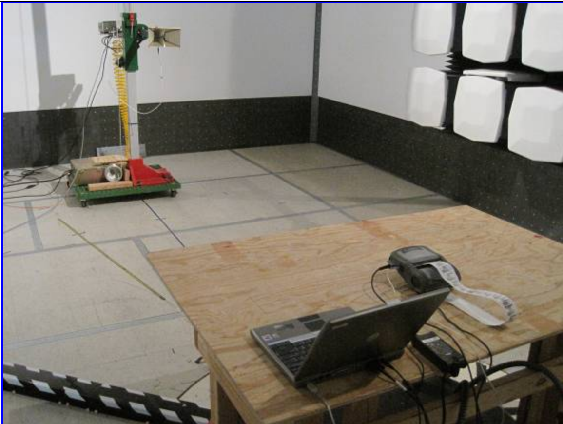
Host: QL 420plus Radiated Emission Test Setup – Rear View
