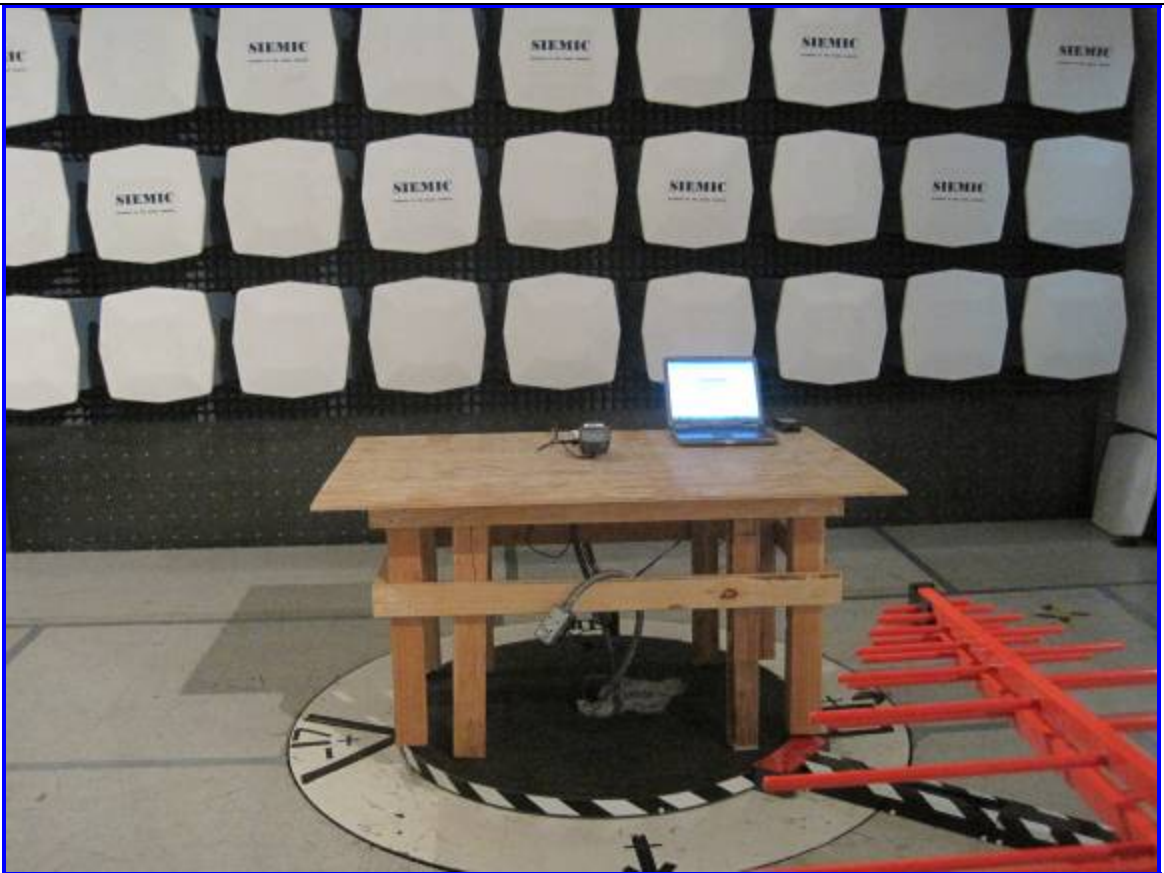
Host: QL 220plus Radiated Emission Test Setup – Front View
