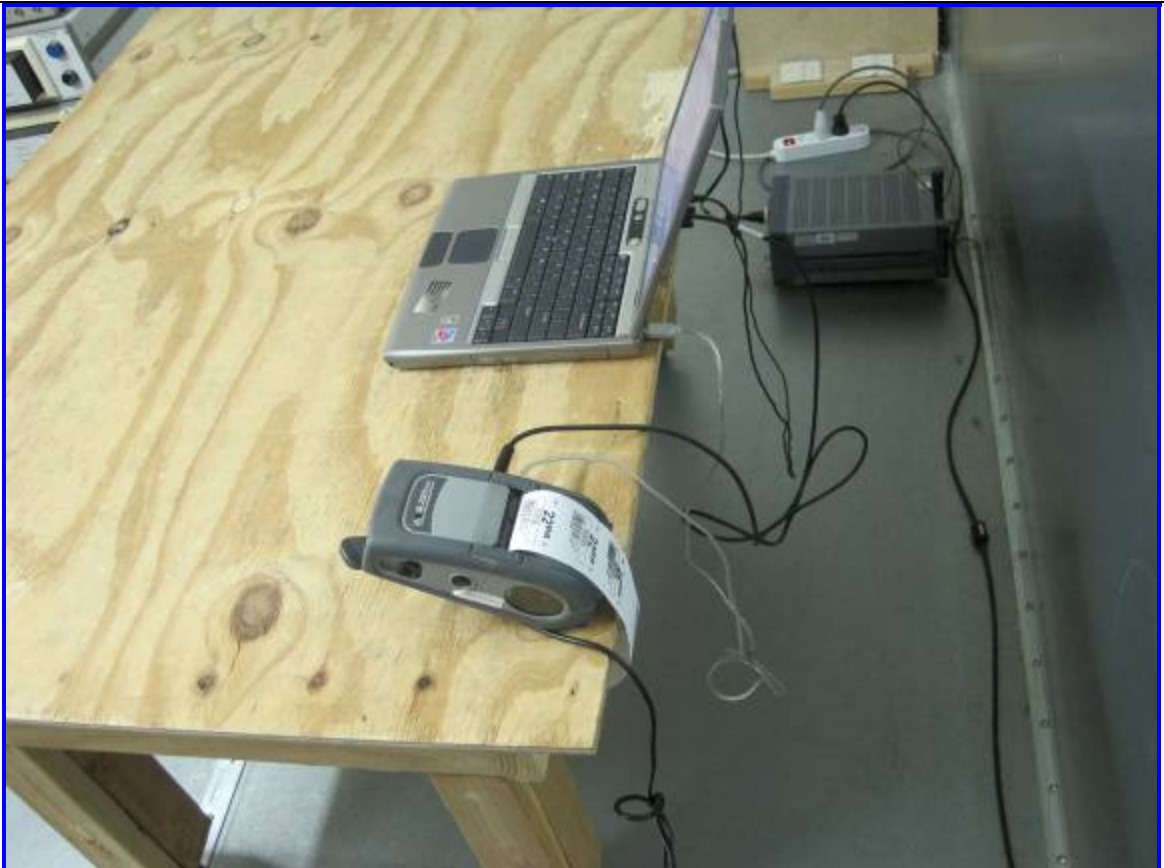
Host: QL 220plus Conducted Emission Test Setup – Rear View
