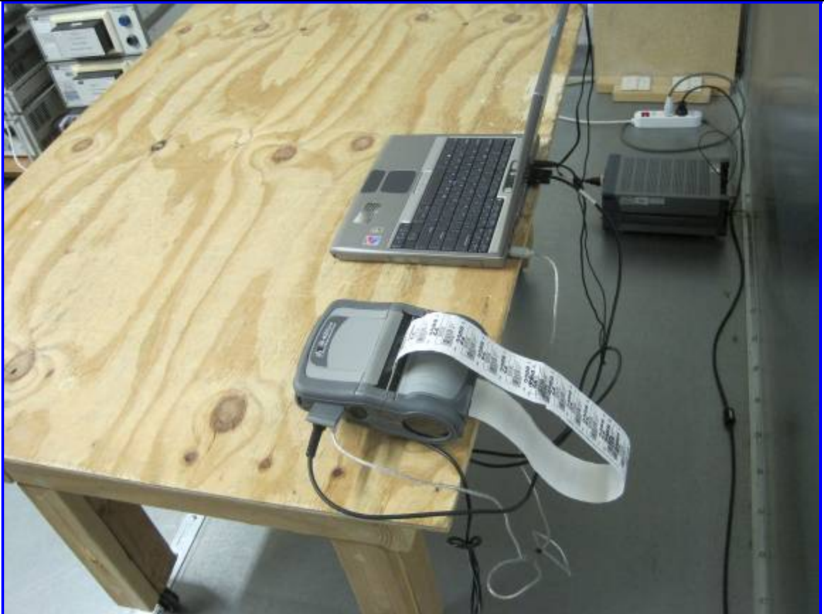
Host: QL 420plus Conducted Emission Test Setup – Rear View
