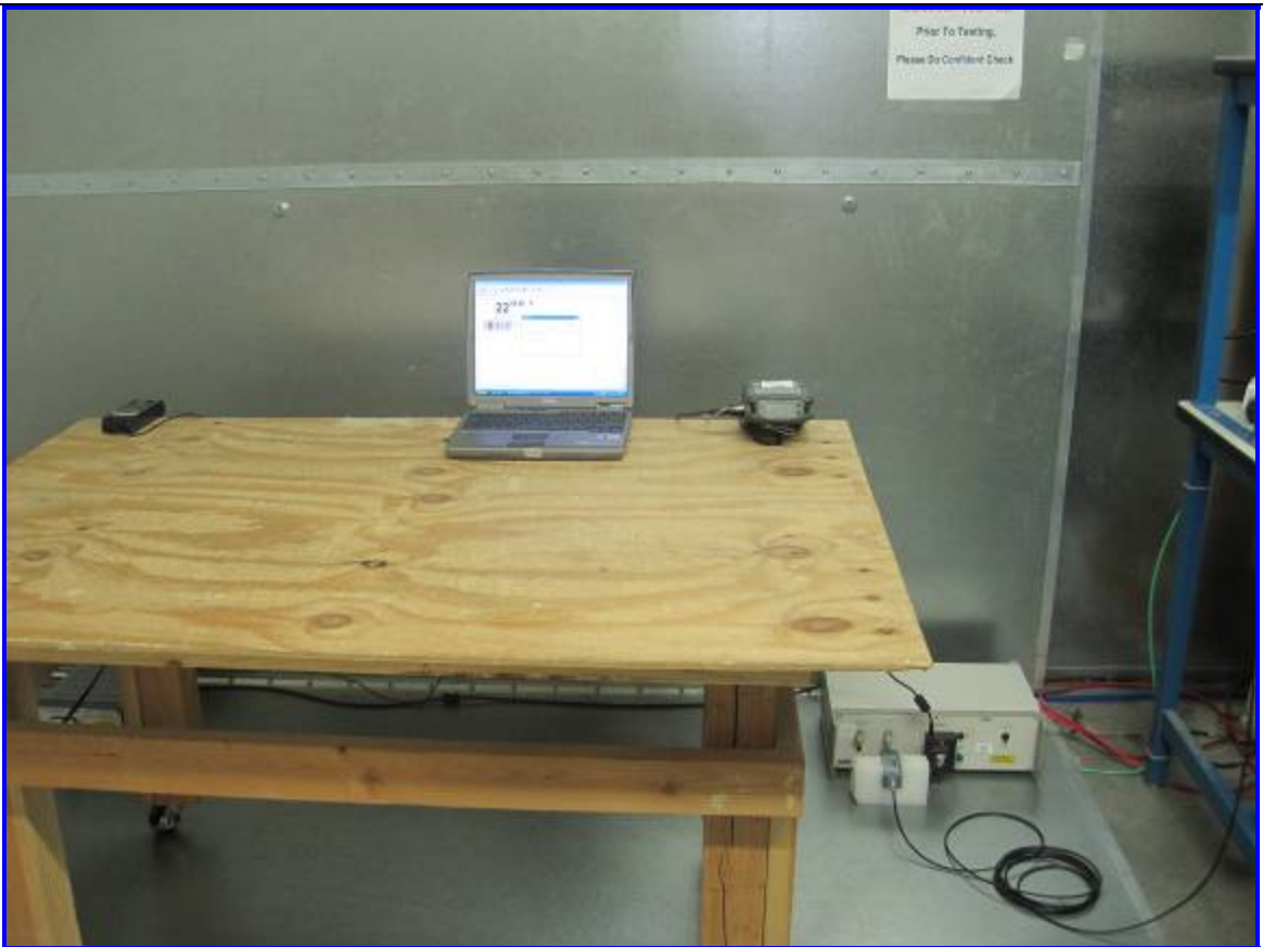
Host: QL 320plus Conducted Emission Test Setup – Front View
