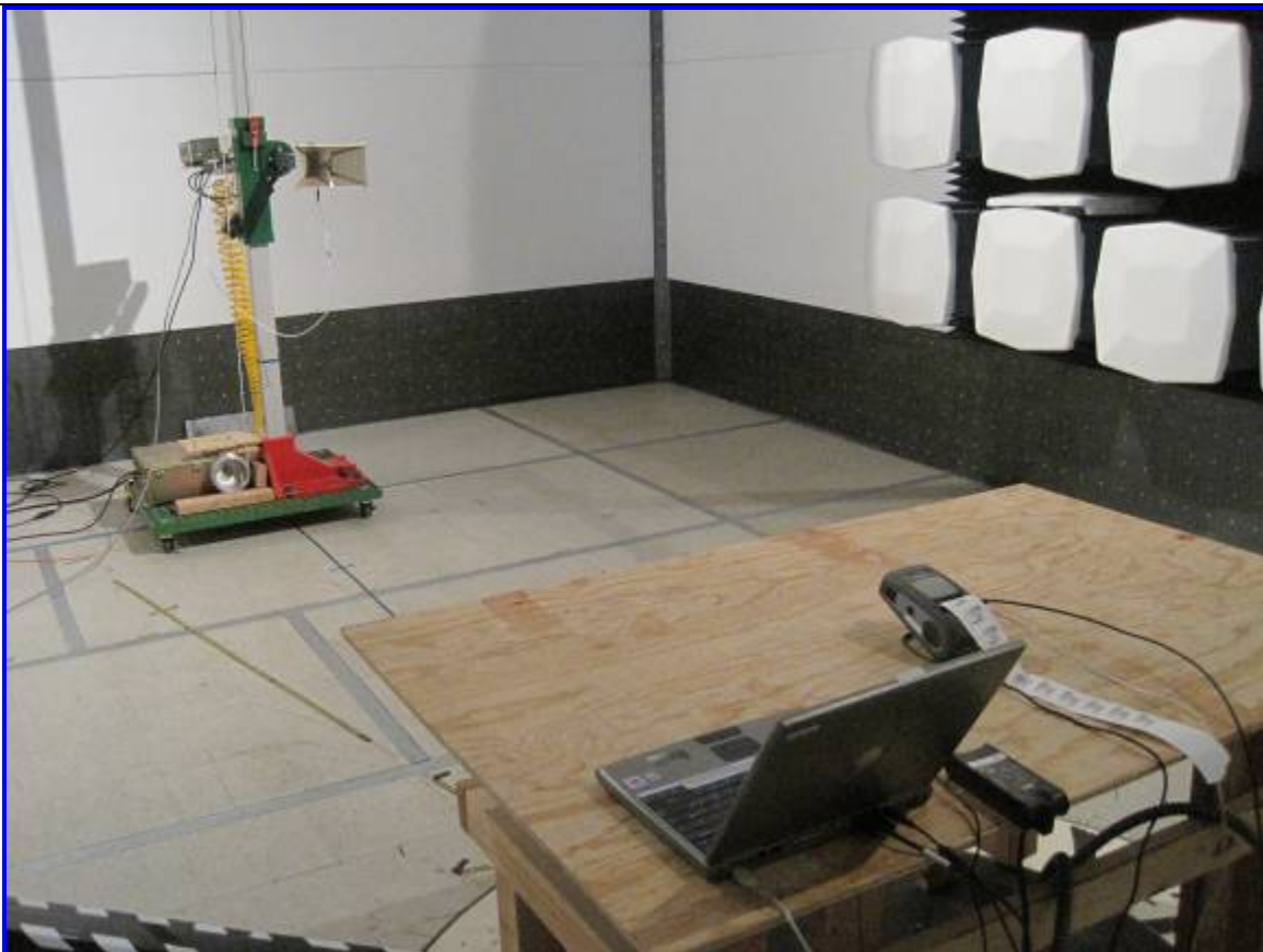
Host: QL 220plus Radiated Emission Test Setup – Rear View
