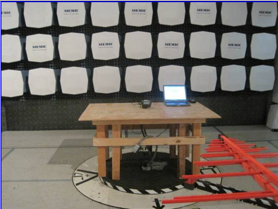
Host: QL 320plus Radiated Emission Test Setup – Front View
