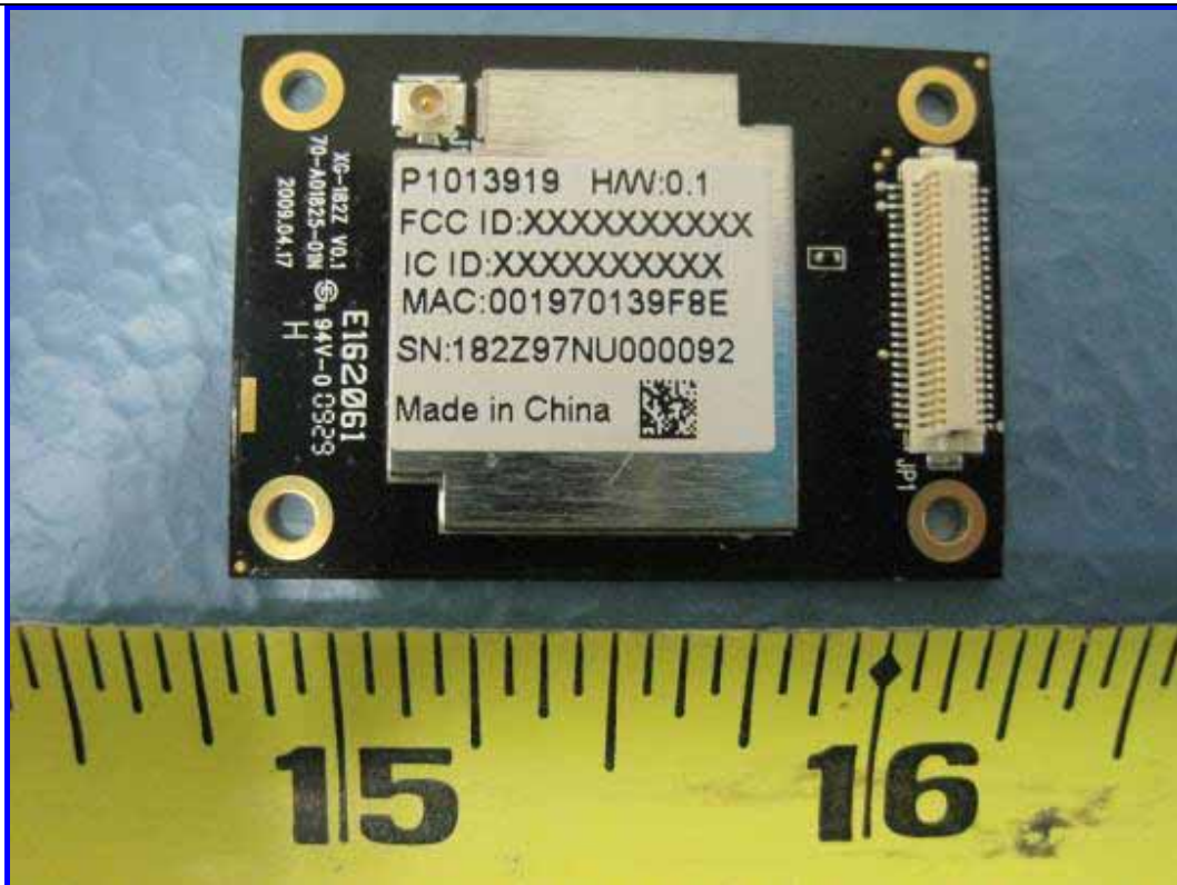
EUT RF Module with Cover On View
