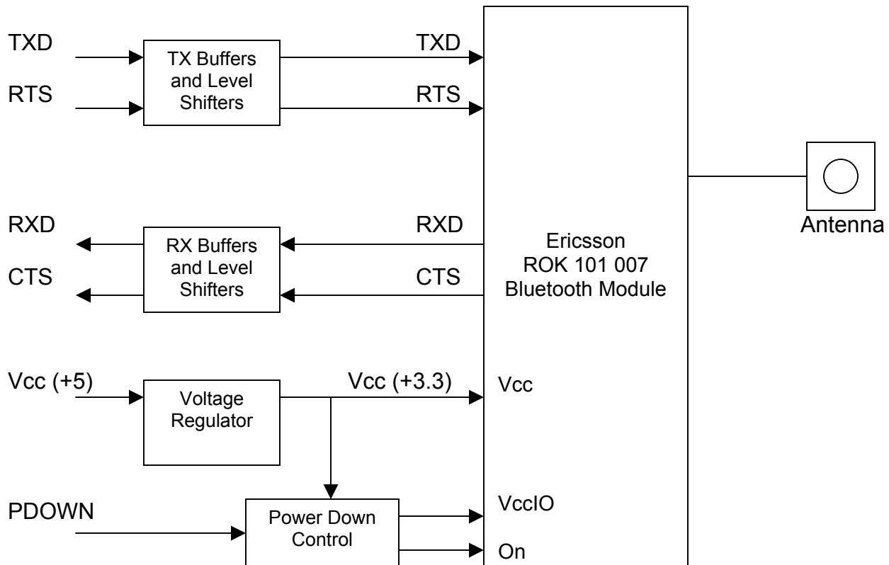
The CC15727-1 module digital interface is at 5-volt CMOS levels. The Ericsson ROK 101 007 module digital interface is at 3.3-volt CMOS levels. All inputs to the CC15727-1 module are buffered. Additional buffering is present at the inputs of the ROK 101 007. There is a voltage regulator on the CC15727-1 module that steps down from 5 volts to 3.3 volts. There is additional voltage regulation on the ROK 101 007 module. The Ericsson module is self-resetting at power-up.
