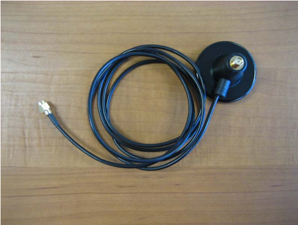
External Antenna Port with coaxial cable
