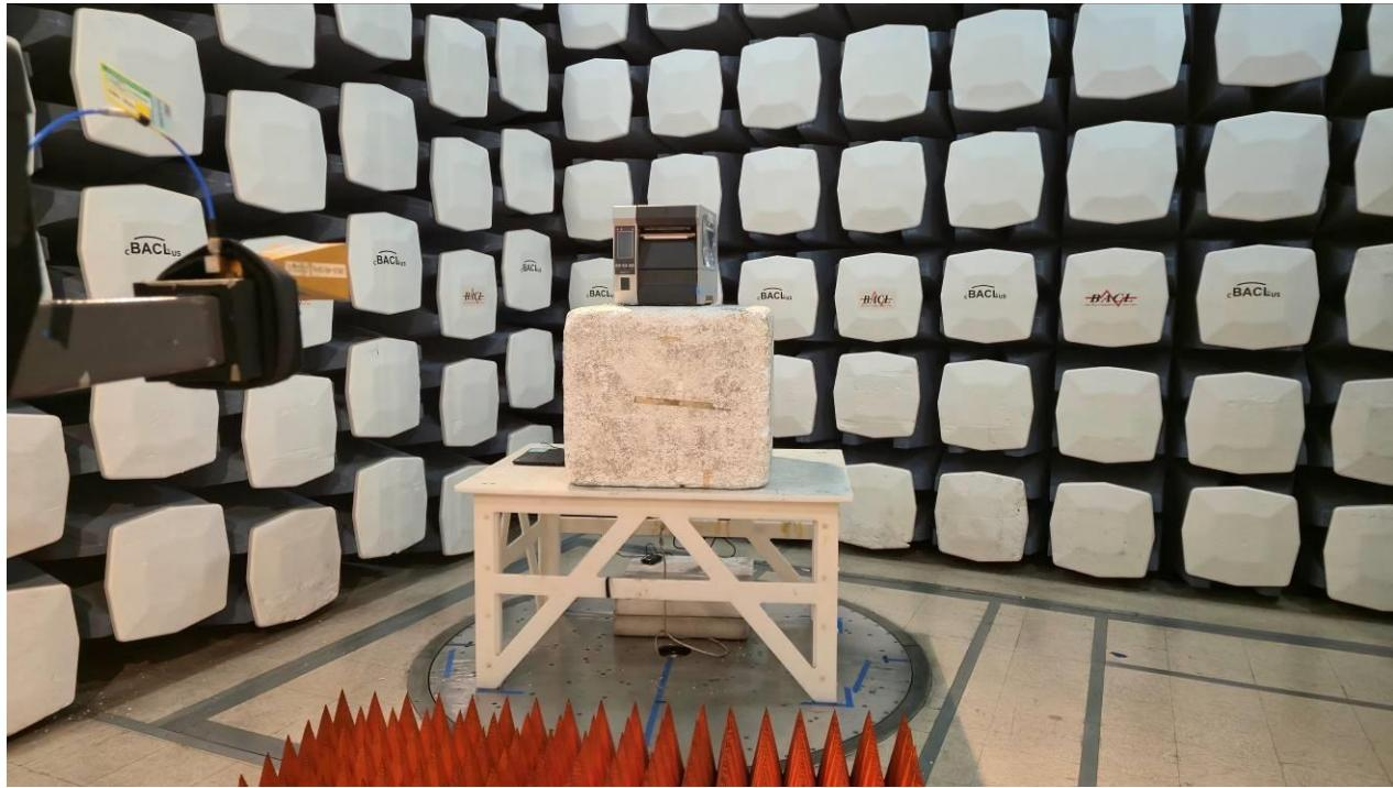
**1.10 Radiated Spurious Emissions: 26.5 GHz to 40 GHz, Rear View at 3 meters distance**
