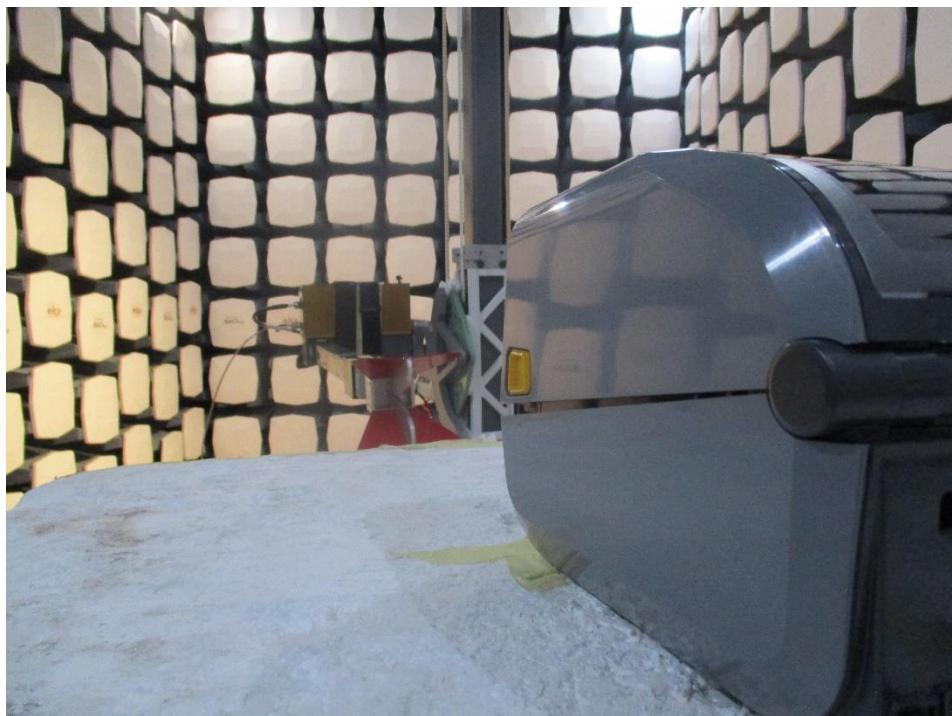
**1.5 18 – 26.5 GHz at 1 Meter Front View**
