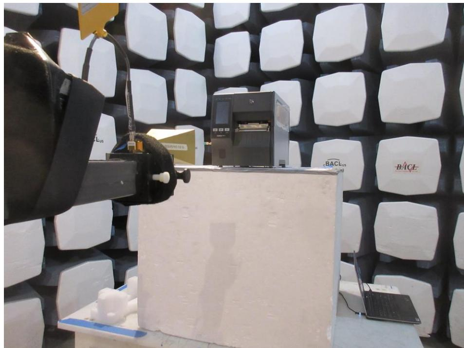
**1.6 Radiated Spurious Emissions measured at 1 meter, 18 GHz to 26.5 GHz, Rear View**
