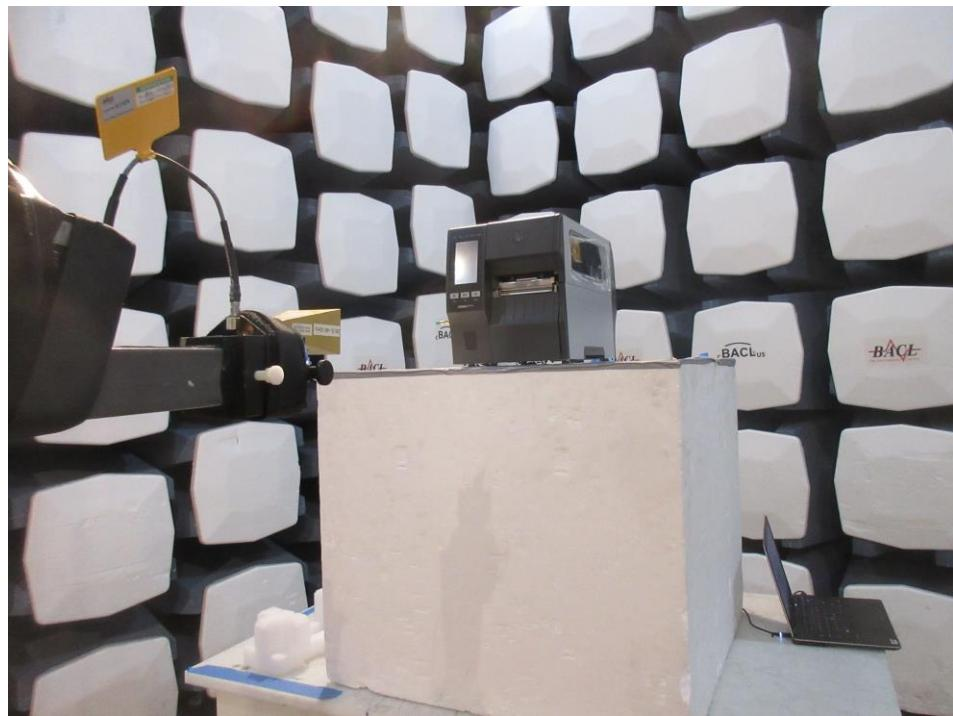
**1.8 Radiated Spurious Emissions measured at 1 meter, 26.5 GHz to 40 GHz, Rear View**
