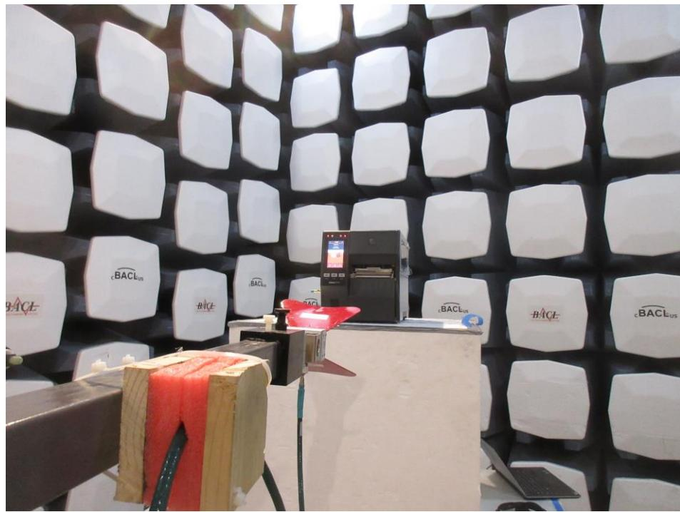
**1.4 Radiated Spurious Emissions measured at 1 meter, 1 GHz to 18 GHz, Rear View**
