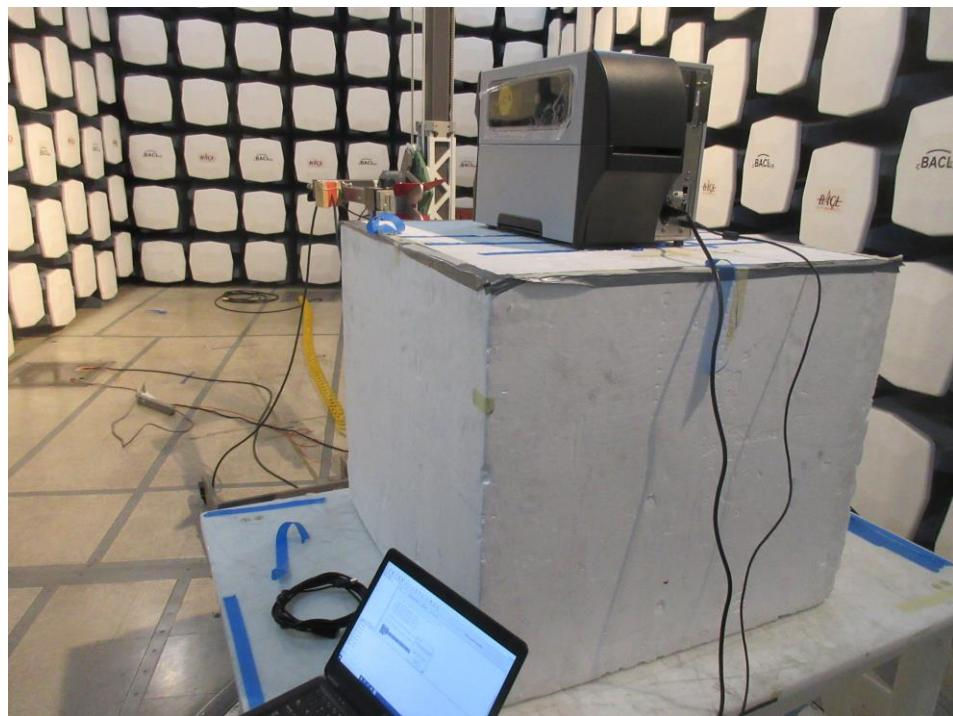
**1.5 Radiated Spurious Emissions measured at 1 meter, 18 GHz to 26.5 GHz, Front View**
