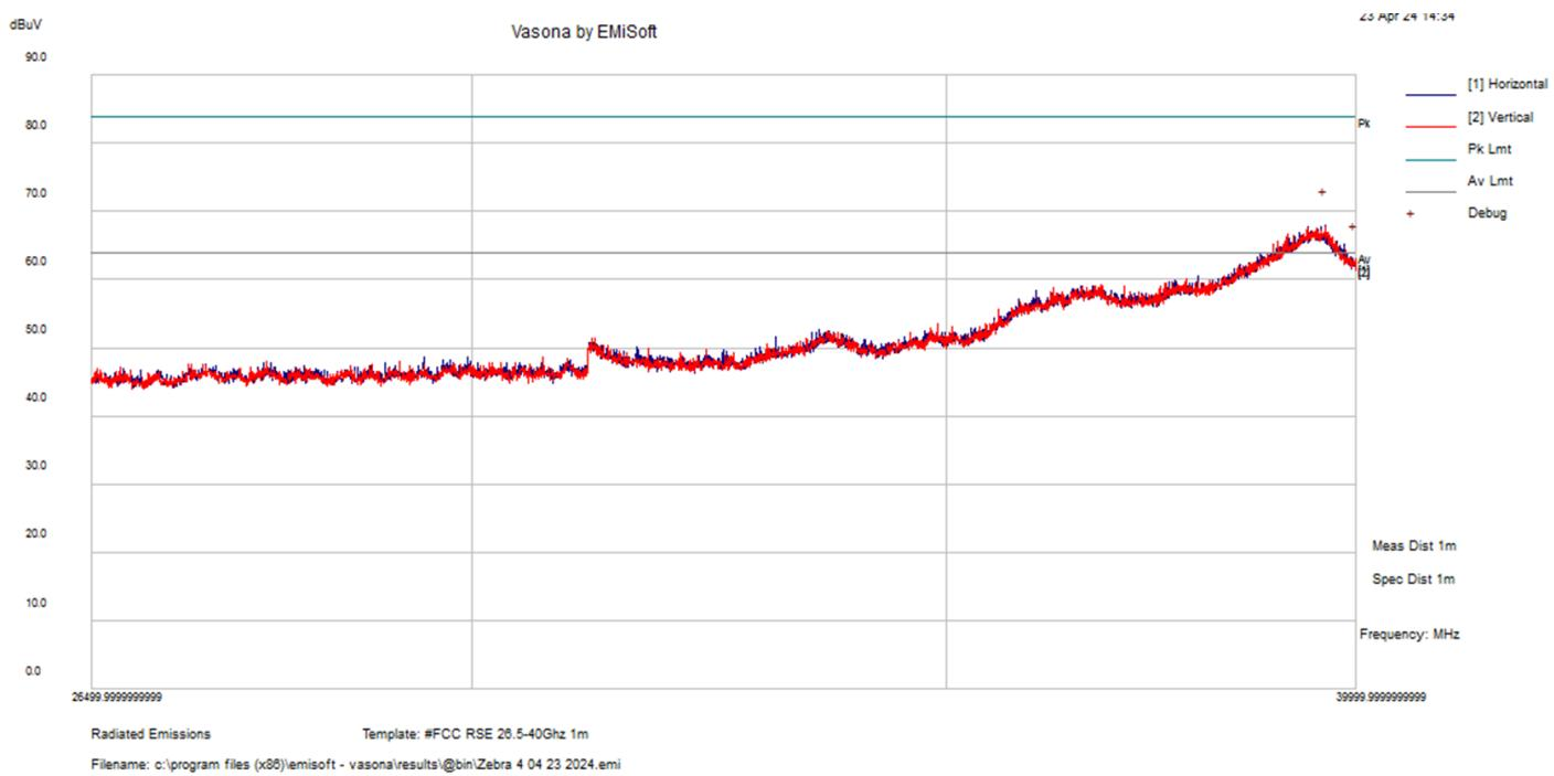
**Note: Above plot shows peak emissions pass under average limits for emissions under 39GHz. For emissions above 39GHz refer to following plot.**
