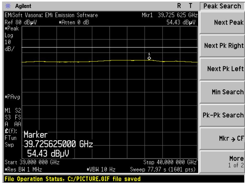
**Note:** above plot shows reduced VBW to make average measurements comparing to average limits and thus show compliance in range of 39-40GHz
