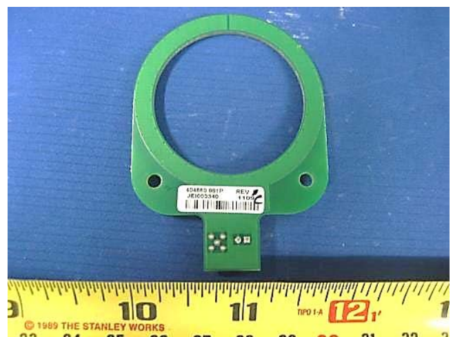
Antenna 1 Bottom View
