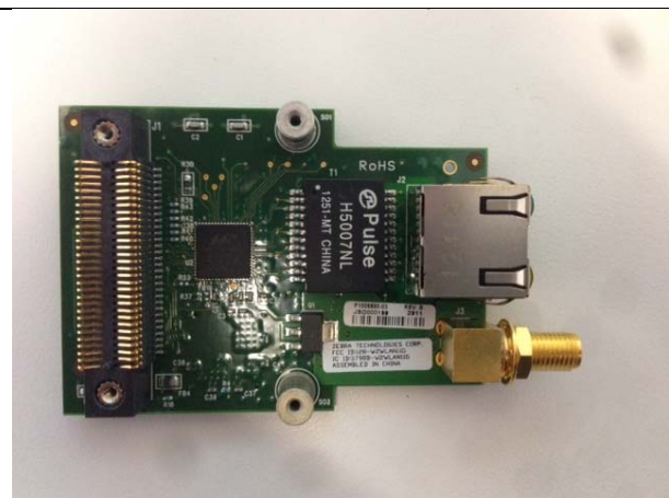
WLAN Radio Board Top View
