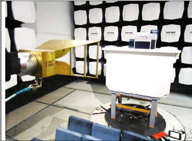
Radiated Emissions (>1GHz) – Front View
