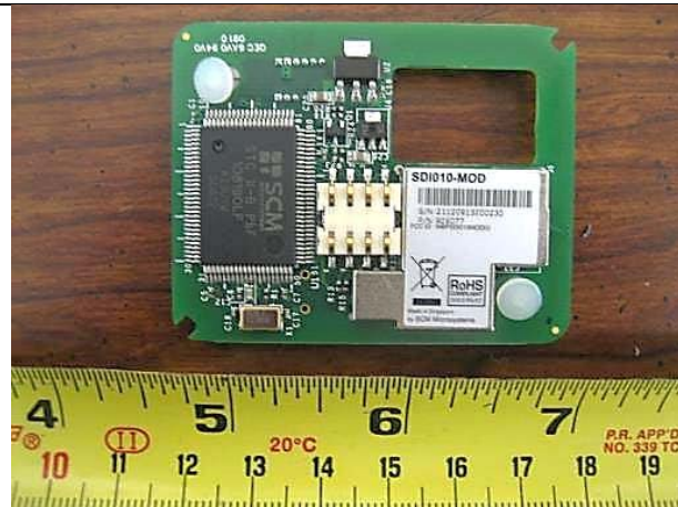
PCBA6 with Shielding Top View
