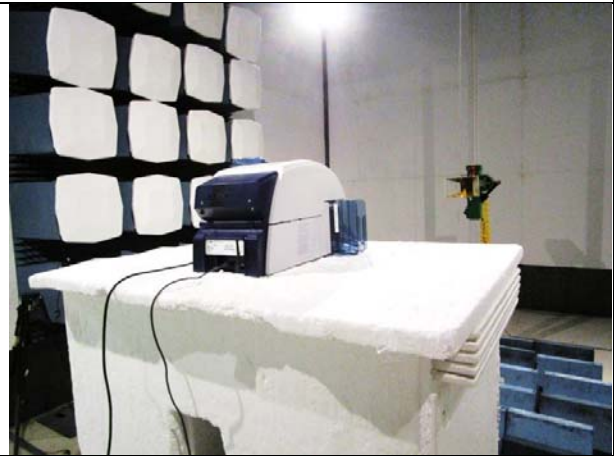
Radiated Emissions (>1GHz) – Rear View
