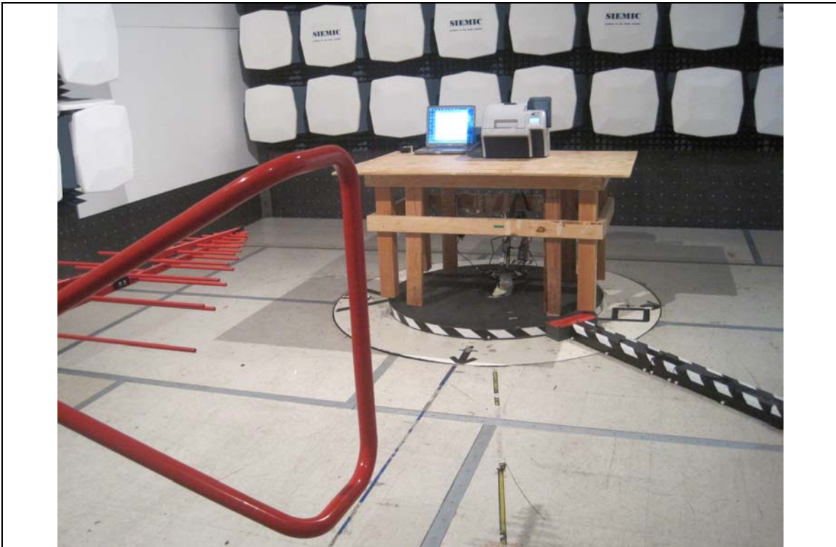
Radiated Emission Test Setup (below 1GHz) - Front View
