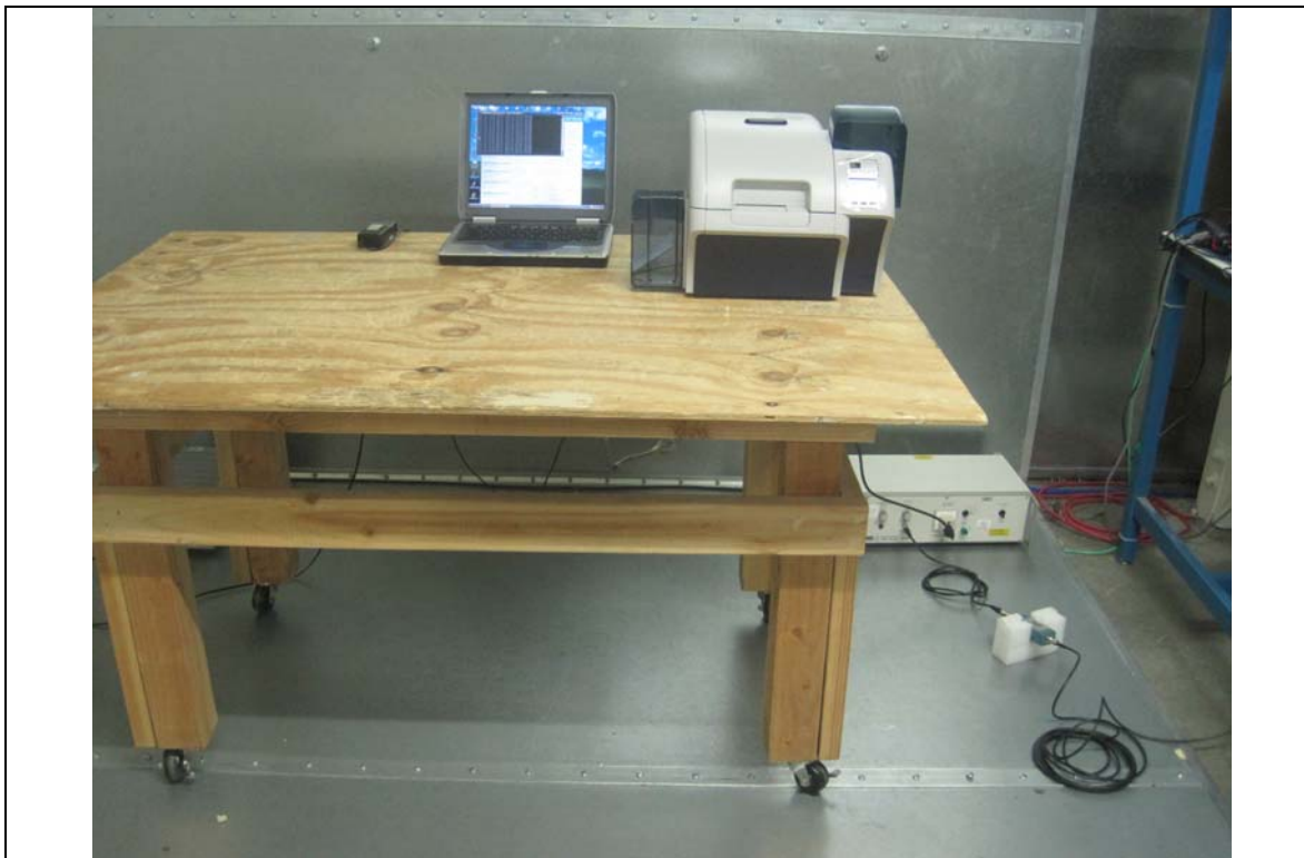
Conducted Emission Test Setup – Front View
