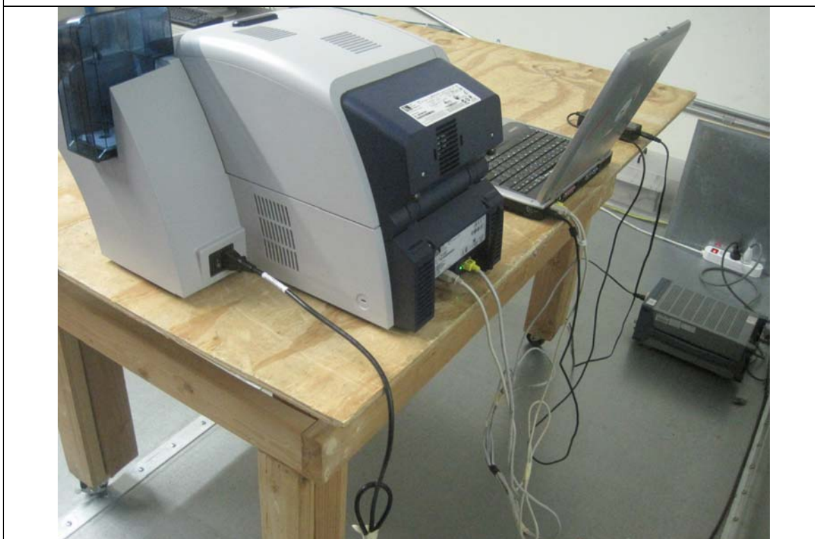
Conducted Emission Test Setup – Rear View
