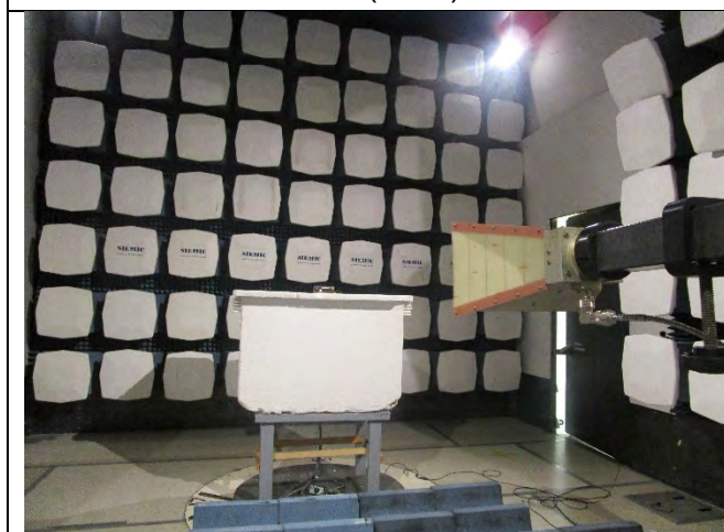
Radiated Emissions (>1GHz) – Front View
