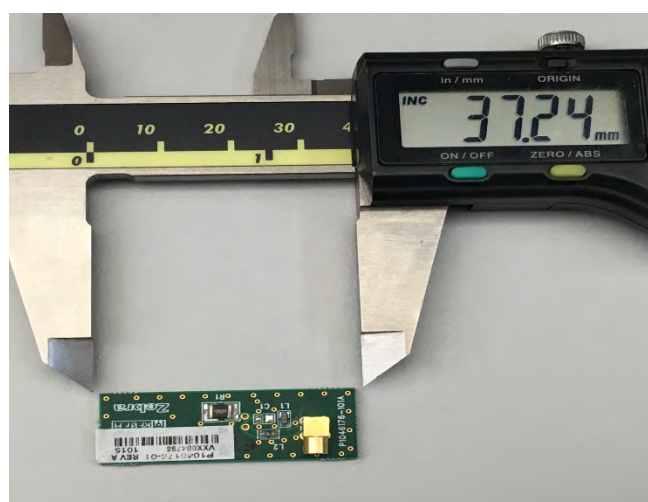
RFID Antenna Top View
