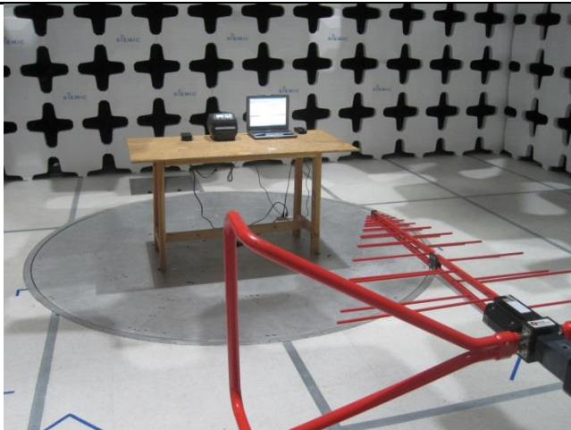
Test setup at 3 meter distance (<1GHz) - Front
