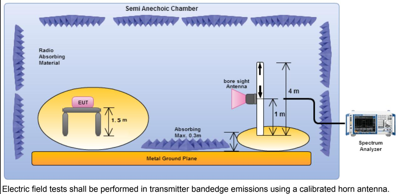
Electric field tests shall be performed in transmitter bandedge emissions using a calibrated horn antenna.
