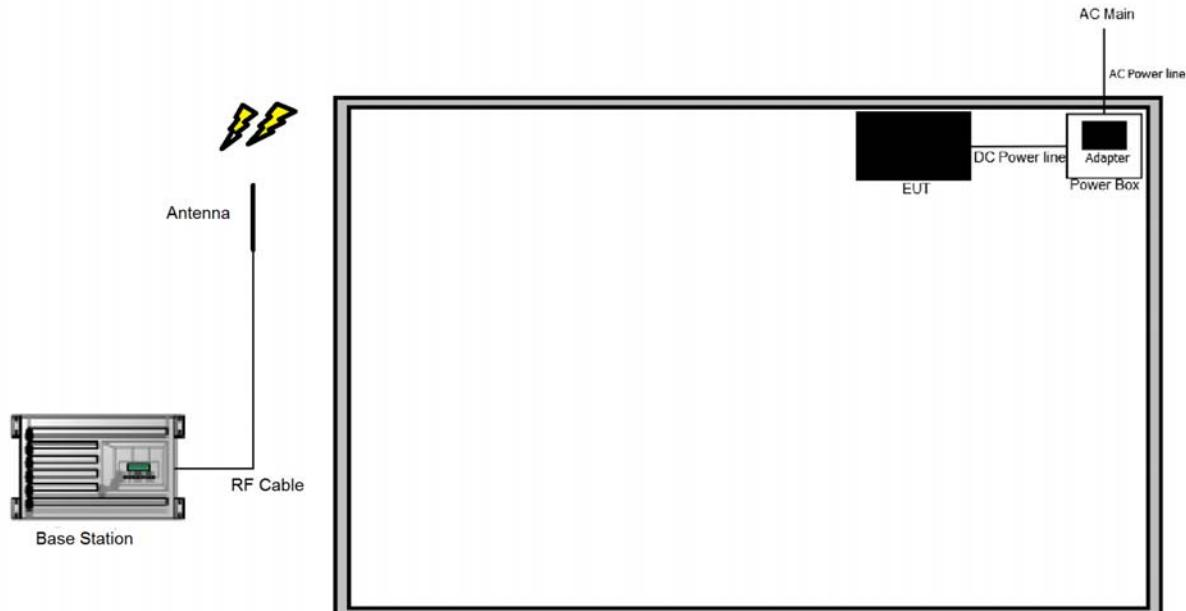
**Test Setup Diagram - Radiated Test**
