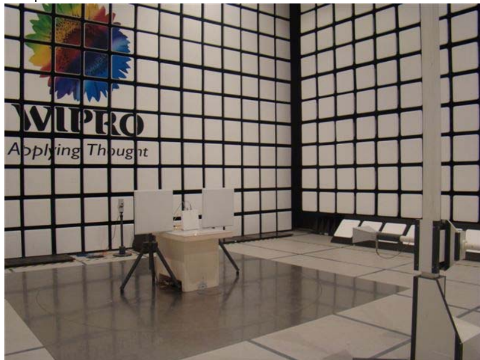
Setup for Radiated Emission
