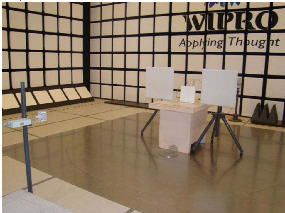
Setup for Radiated Emission
