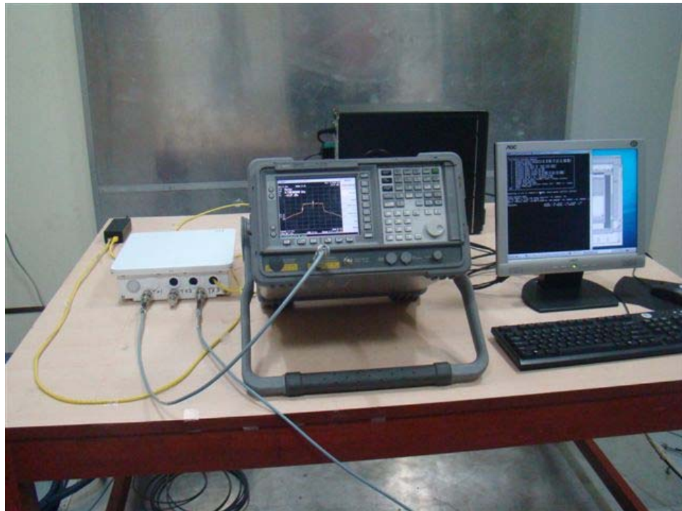
Setup for Conducted measurements
