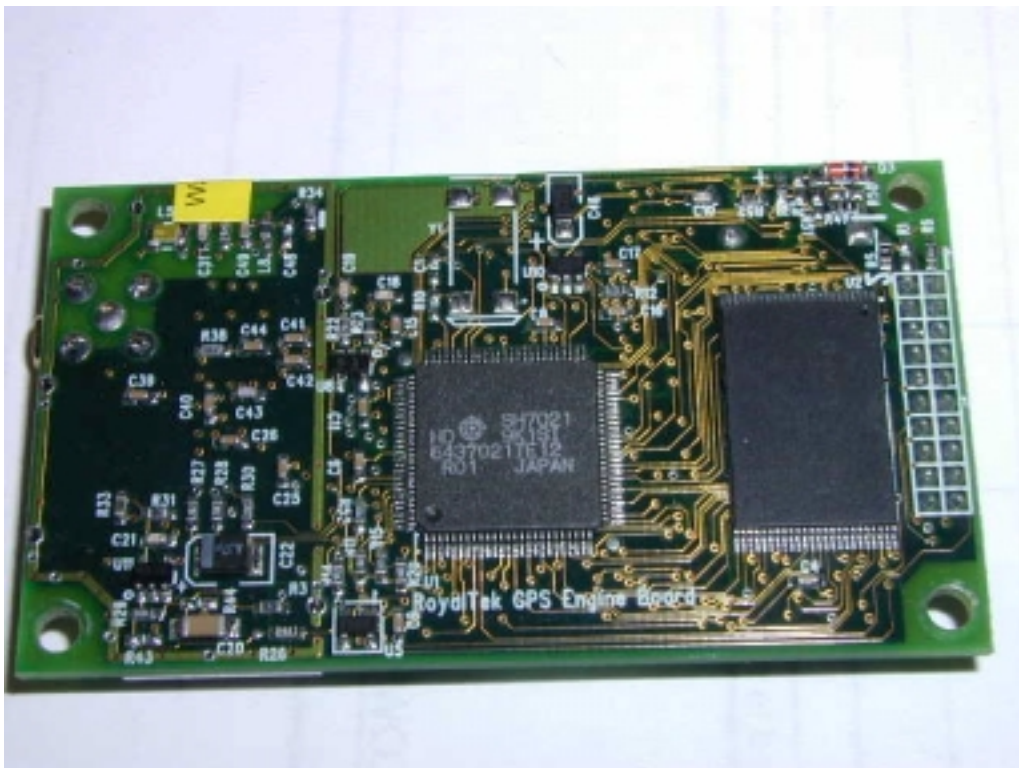
GPS receiver board, side 1 (above).
