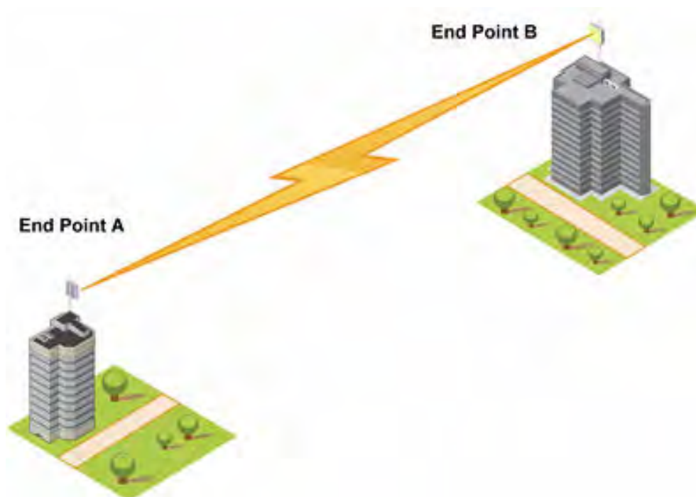
Figure 1-1 Wireless Network Topology (Point-to-Point-Link)
