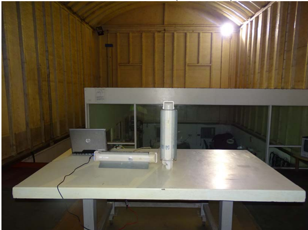
Back View of Radiated Test (Sector Antenna)
